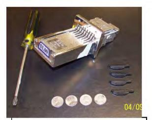
1) Remove the Push Chute from the coin door, and remove the push chute end, proximity plate, anything bolted to the end— for easier access. You will need the Push Chute (of course), enough coins to make it work in its current setting, the inserts for the desired setting, and a Phillips screwdriver.
