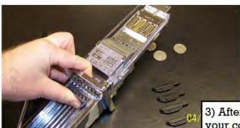
3) After pushing in the chute and your coins drop out, you will be able to access the inserts, and a section that may contain spare inserts. Continue to hold the handle in as shown...
