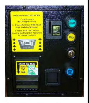
After entering program mode, most of your programming will be done using the buttons mounted on the coin door.
