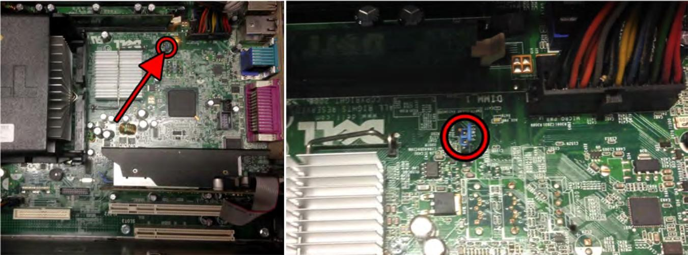
3. Remove the “password reset” jumper.
