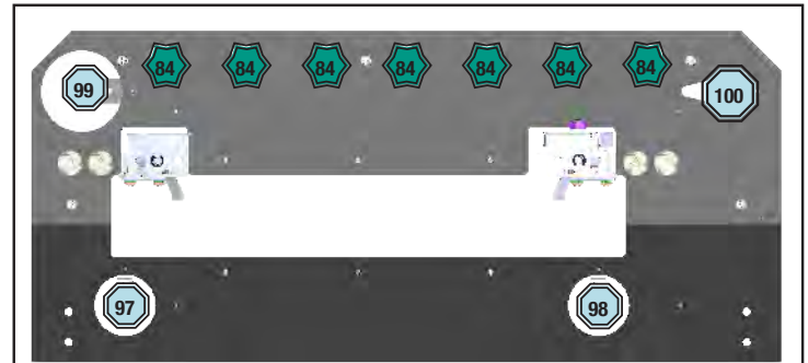
Figure 4.8.1. Back panel detail for Upper Mini Playfield 4-driver 48V Node 10 connections.
