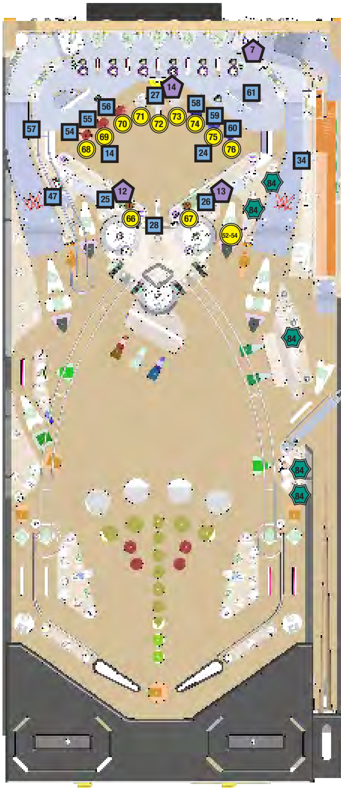
Figure 4.8.2. Upper Mini Playfield 4-driver 48V node 10 playfield location and relevant lighting, switches, and drivers.
