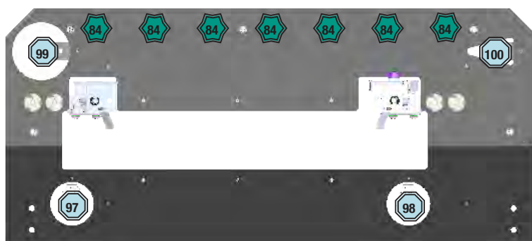
Figure 3.2.5. Playfield back panel lighting locations.
