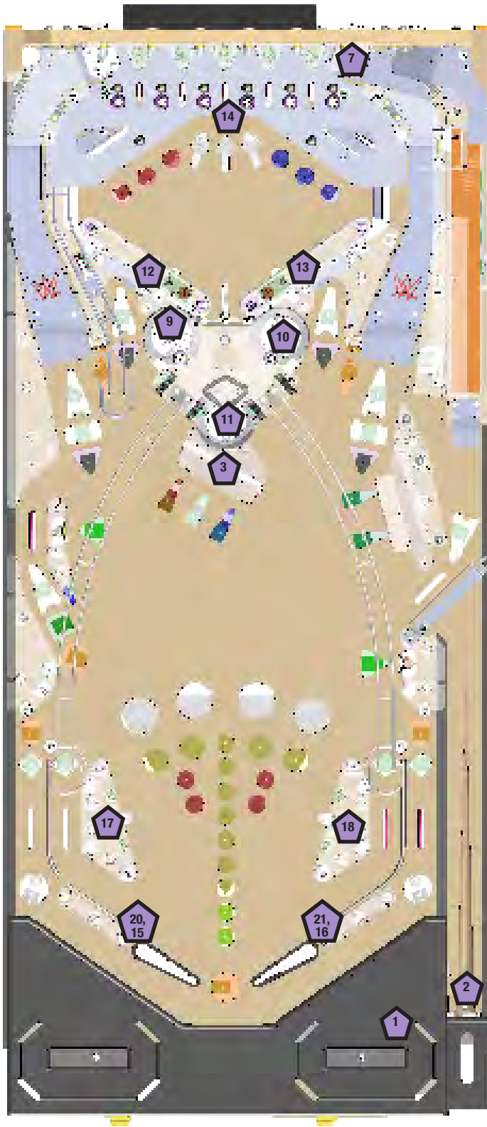
Figure 3.1.2. Playfield top component view
