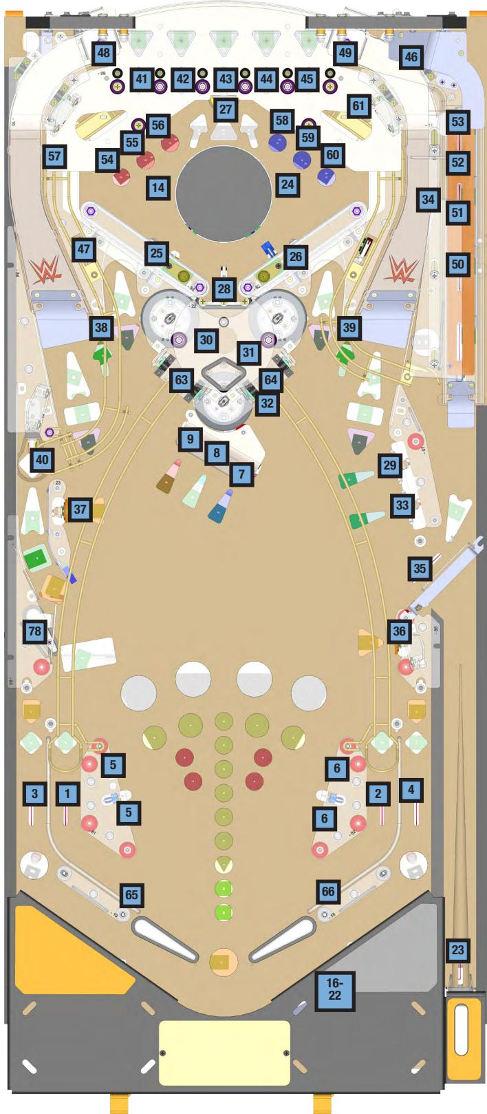
Figure 3.4.1. Switch locations, playfield top view
