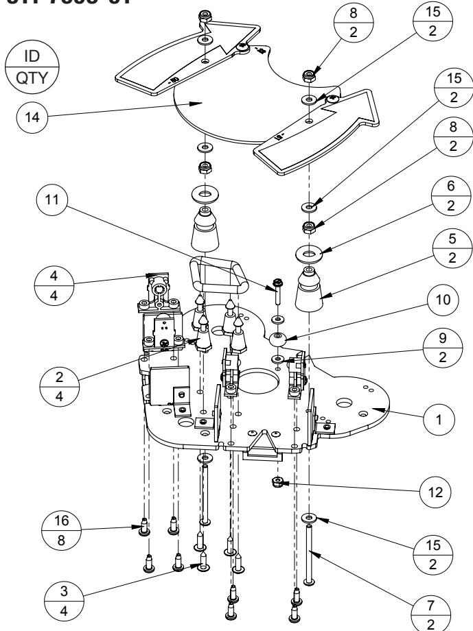
Figure 5.34.3. WWE Pop Bumper Playfield Assembly LE Diagram
