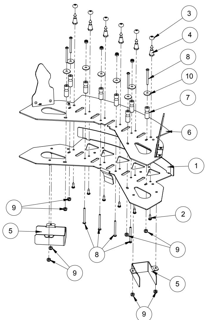
Figure 5.29.1. WWE Top Lanes ASSY LE 511-7620-01 Diagram
