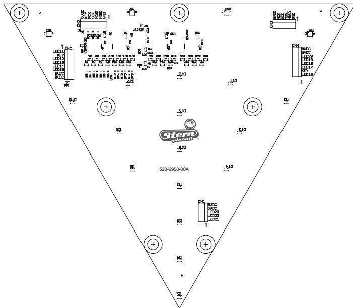
Figure 4.4.1. Lower Playfield LED Board, Connector-side view.
