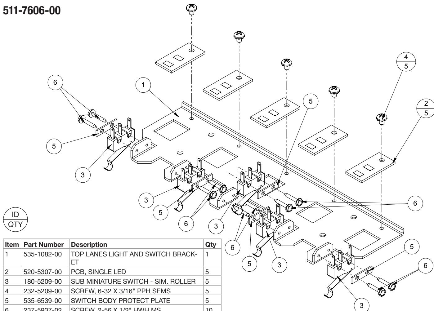
Figure 5.26.1. 511-7606-00 Top Lanes Lights and Switches
