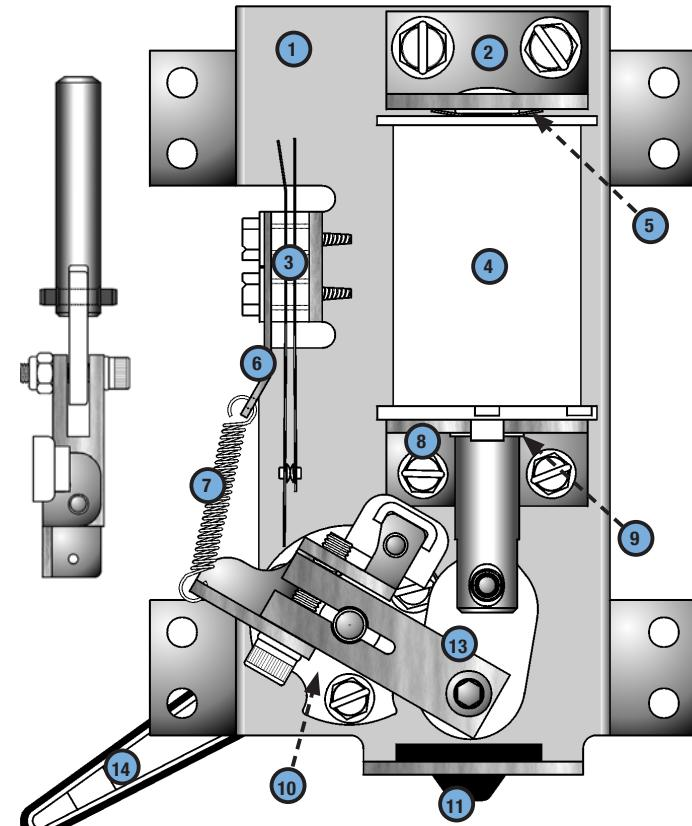
Figure 5.14.2. Right flipper assembly 500-6543-12-ND bottom view.
