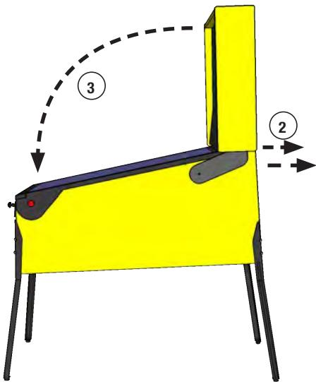
2. Remove the backbox securing bolts
