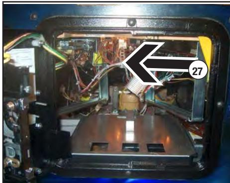
27. Reach inside the cabinet and move and hold the yellow top molding lock handle to the left.
