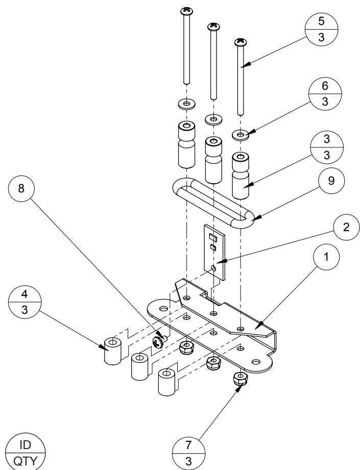
Figure 5.29.3. WWE Pop Bumper Flasher Assembly 511-7627-00 Diagram
