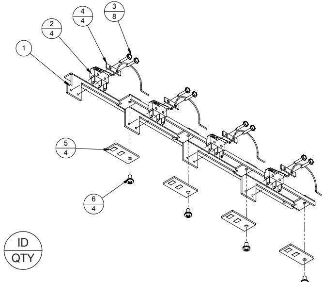
Figure 5.31.1. WWE Ladder Light and Switch Assembly LE Diagram
