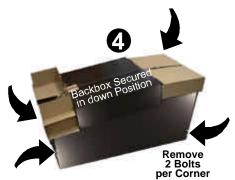
4. At this point DO NOT CUT STRAPPING (You want to keep the Backbox secured in the down position). Loosen and remove the 8 Leg Bolts (use 5/8" Socket Wrench) and set aside.
