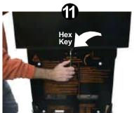
After the BACKBOX is in the UPRIGHT POSITION, locate the 5/16" HEX KEY. While inserted, rotate KEY with a 3/4 turn until latched & locked.
