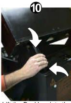
Lift the Backbox into the UPRIGHT POSITION (Ensure the cables do not get pinched).
