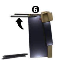
6. Install FRONT LEGS using the bolts removed from Step 4. Secure tightly. Take care not to scratch the Black Finish on any of the Legs.
