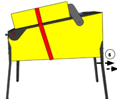
2. Remove the backbox securing bolts
