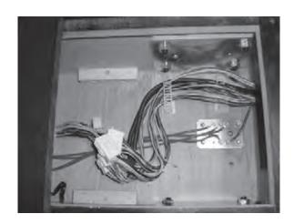
Fasten the cable down with the 3 cord clamps.
