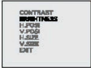
(3) Press the SET button (to decide selection). When the selection of the BRIGHTNESS adjustment mode is decided, the adjustment data scale bar appears on the screen.
