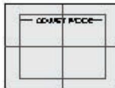
Make adjustment so as to have red superimposed on green. When red is superimposed on green, the color becomes yellow.
