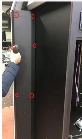
13. Remove the speaker cover and beam support plate from the L/R light box.
