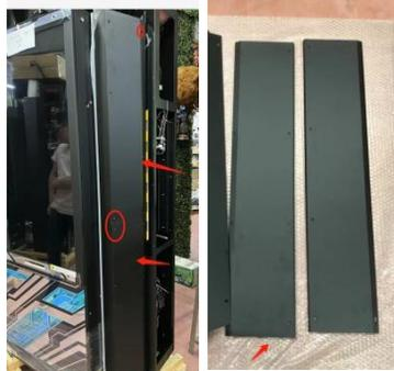
8. Remove the R side frame assembly
