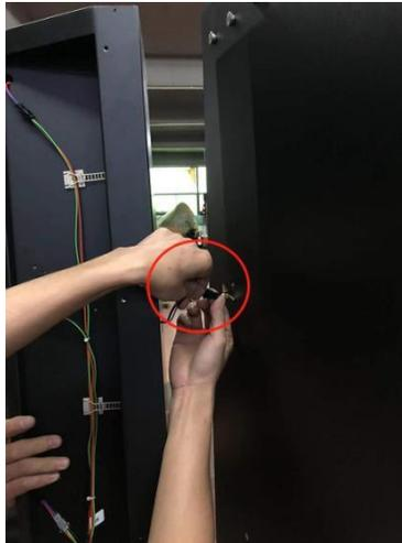
10. Hang the L/R side frame on the monitor cabinet and fix it with 5 screws.
