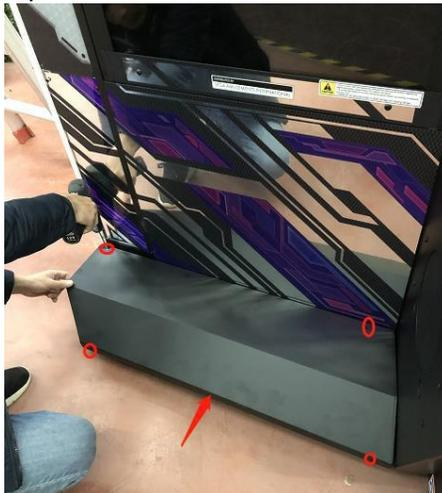
34. Connect the start button wire and fix the console panel to the console frame with screws.
