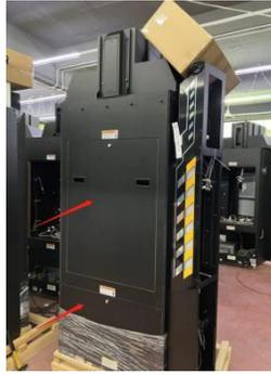
12. Remove the beam assembly (**Be caution with the gun assembly!**)
