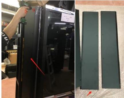
10. Remove the L side frame assembly
