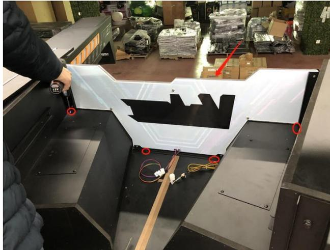
28. Fix the LED plate to the light box and connect the LED wire.
