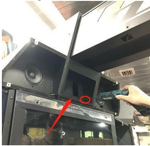
22. Connect the speaker LED wire and fix the speaker cover to the light box.
