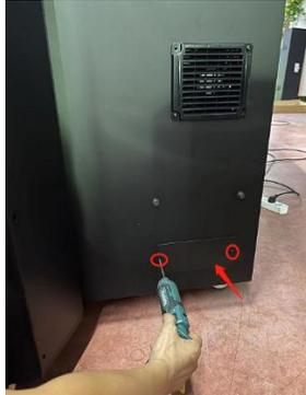
31. Fix anchors to the L/R pedal.
