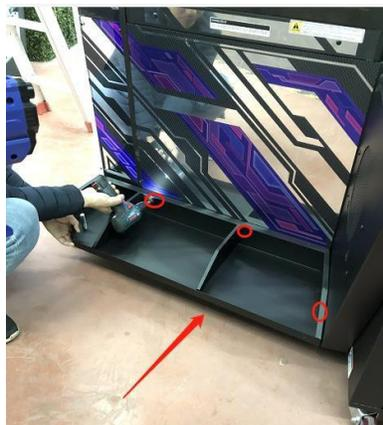
33. Fix the L/R pedal cover to the pedal
