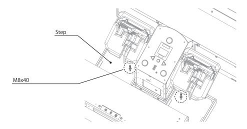
Place the Floorboard on the Step. One person should continue supporting the Floorboard until step 8.
