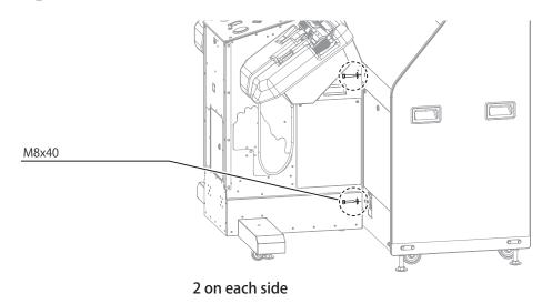
Remove the 2 screws and remove the Side Lid.
