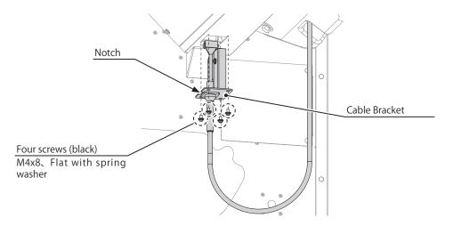
Remove one screw and remove the cable bracket from the Controller When installing, refer to "How to attach cable bracket" below
