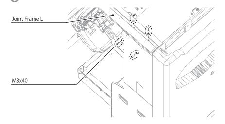
Temporarily fix the Joint Frame L to the Monitor Cabinet with 4 hex bolts.
