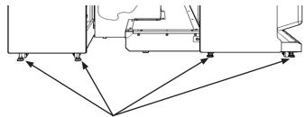
Each leg adjuster MUST be lowered so that the casters are raised approximately 5mm off the floor
