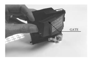
Open the reject gate to gain access to the rundown path.
