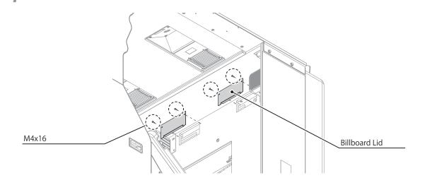
Insert the Billboard Plate into the Billboard Box and secure with two truss screws.
