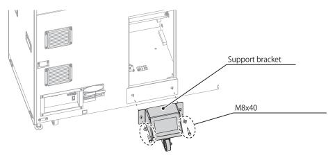
Attach the Support Bracket inside the Cabinet with 2 hex bolts.
