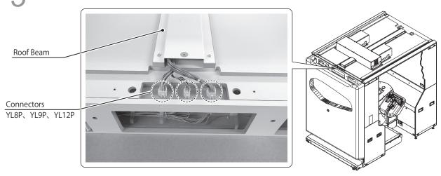
Attach the Connector Lid Seat with 3 screws.
