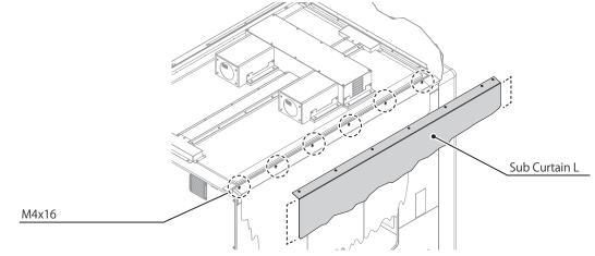
Hook the two Curtain Sashes onto the temporarily fixed truss screw and fully tighten 6 truss screws. At this time, please make sure cutout of Curtain Sash faces outward.
