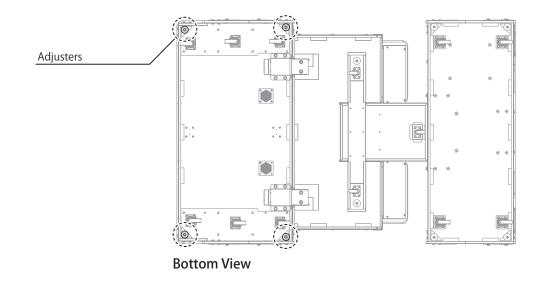
At least two people support the Joint Frame L and place it on both the Monitor Cabinet and Seat Cabinet in the orientation shown.
