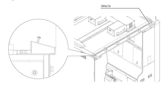
Hook the Side Curtain to the temporarily fixed truss screw.
