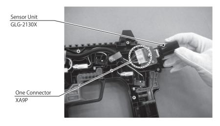
Refer to steps 1 to 3, install the new Sensor Unit in reverse order and reassemble. Be careful not to overtighten the screws.
