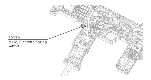
Lift the Controller cable and disconnect connector
