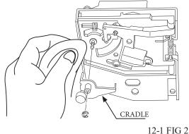
After wiping off as per previous step, further apply a dry cloth to completely dry the Coin Selector.
