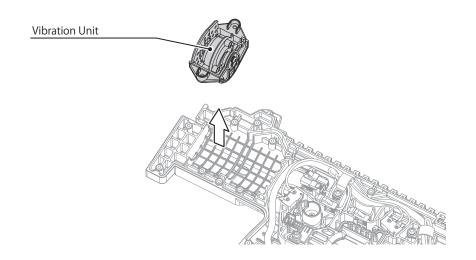
Remove the 2 screws and remove the Controller Vibration Unit.
