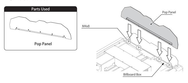
**7** Fully tighten the four screws used in step 1.
