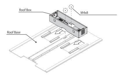
Attach two Roof Box Brackets with 8 screws.
