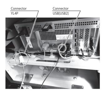
Connect two connectors to the rear of the drive.
