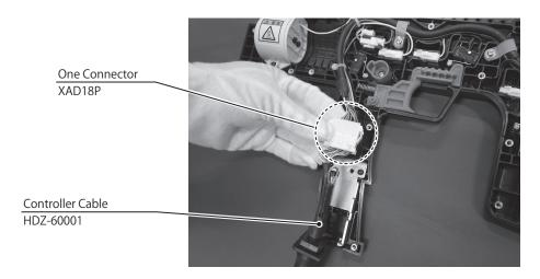
Refer to steps 1 to 4, install the new Controller cable in reverse order and reassemble. Be careful not to overtighten the screw
