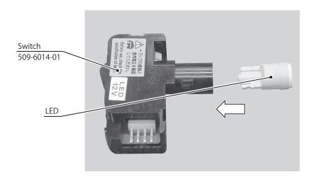
Refer to steps 2 to 4, install the new switch in reverse order and reassemble
