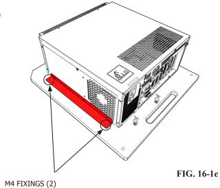
Lift and remove the Game Board from the wooden BASE GAME BOARD. The Game Bd is HEAVY, take care not to clash with other components when removing as this could cause component damage.
