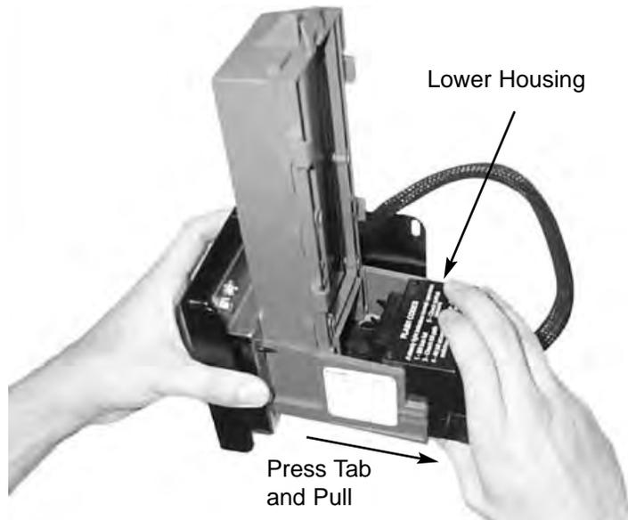
C.) Remove Jam, and reassemble.
