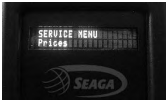
Fig. 10 – LCD Display while in Service Mode. The Prices menu is the first sub-menu.
