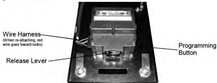
Figure 6 – Removing the Bill Validator
