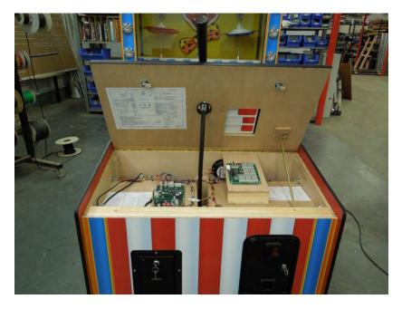
Coin doors – Opening the top door gives access to the coin mechanism, and opening the bottom door gives access to the cash box.
