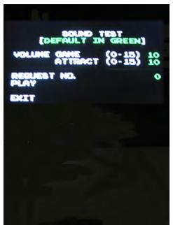
This is provided to allow the owner to set the basic sound level of the attract mode to a different volume level than that used, in normal game play. Caution should be observed when making adjustments so the main volume is not to loud when the volume potentiometer is turned all the way up.
