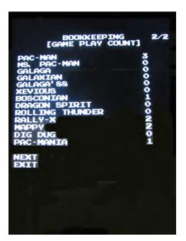
These tables are self-explanatory showing details such as how many times a particular game was played, how long the power was on, and total play time etc. An error log is provided to keep track of discrepancies detected by the processor board that may help a technician in troubleshooting the game should major errors occur later.
