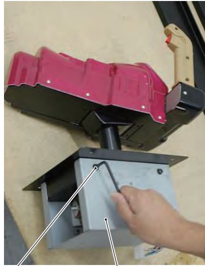
Flange socket bolts (M6 x15) Gun base box
