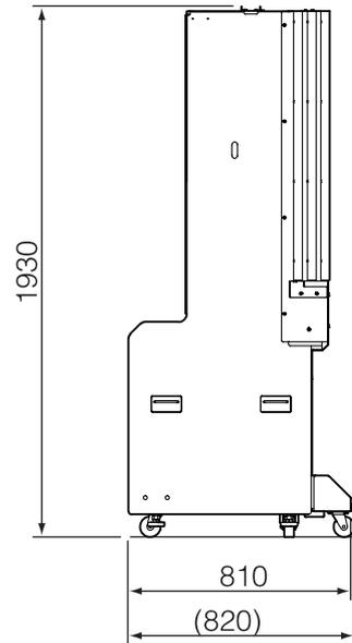
Refer to the above dimensions and check beforehand that the machine can be carried in without problem.
