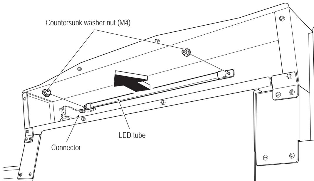
**4** Remove the LED tube caps U and L, and remove and replace the LED module.
