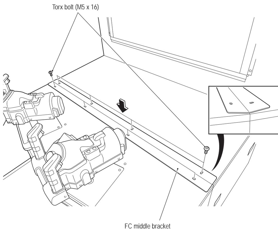
\* There is further assembly work to be performed, so leave the service panel L and service panel R open.
