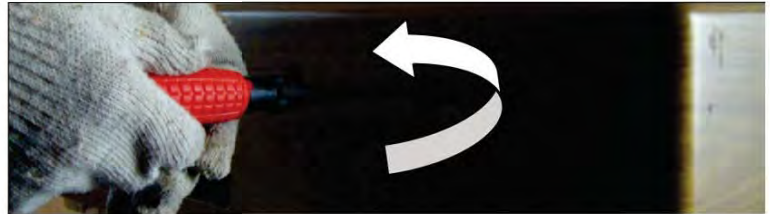
2. Loosen the five Philip screws inside the playing surface
