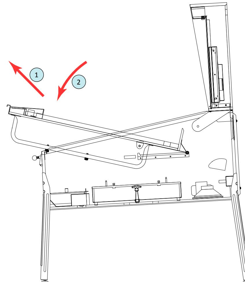
Figure A13. Moving the playfield to position 2.
