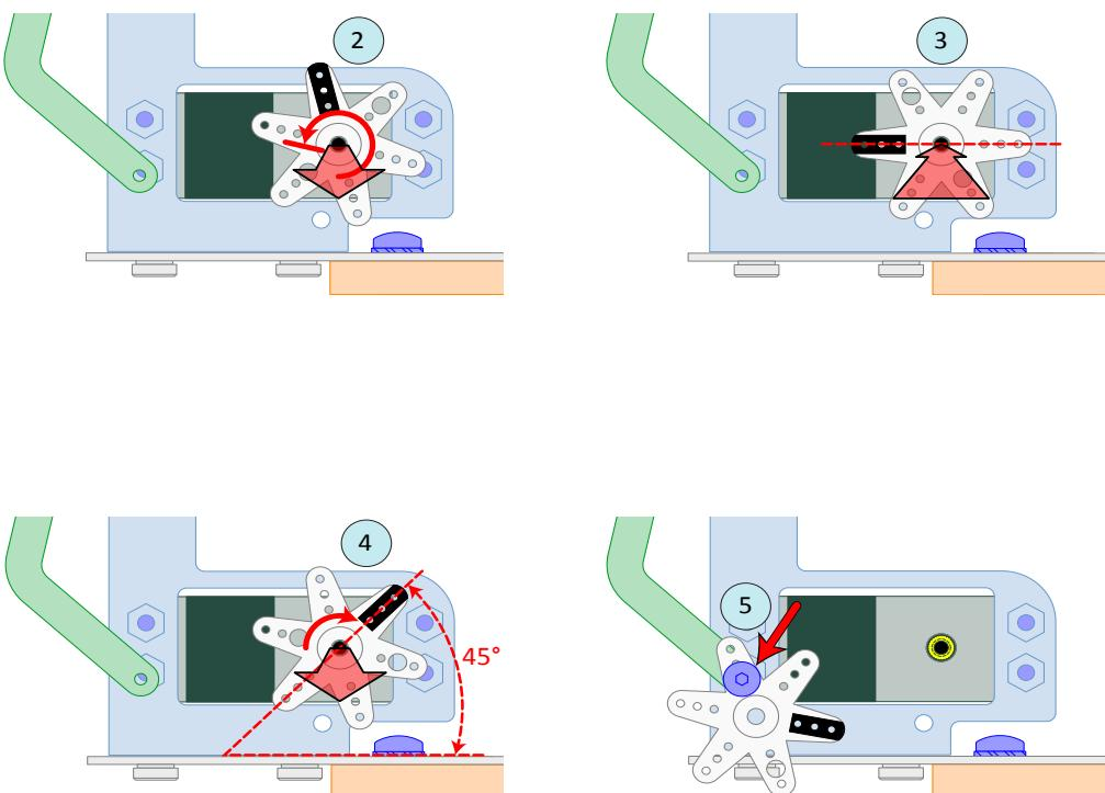
Figure E4. Calibrating the Smaug Assembly servo horn.
