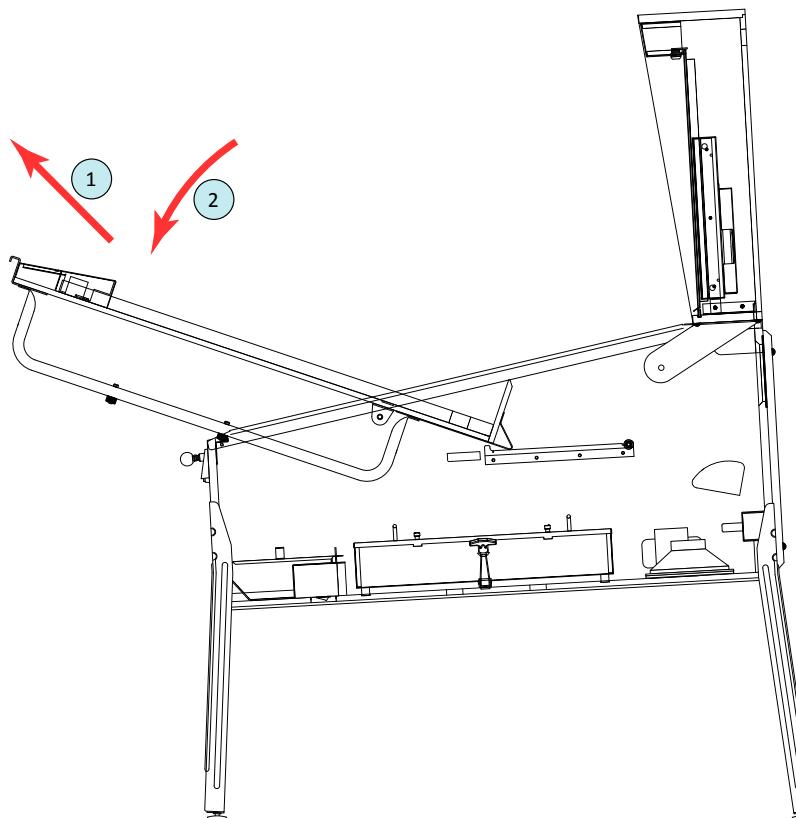
Figure A14. Moving the playfield to position 3.
