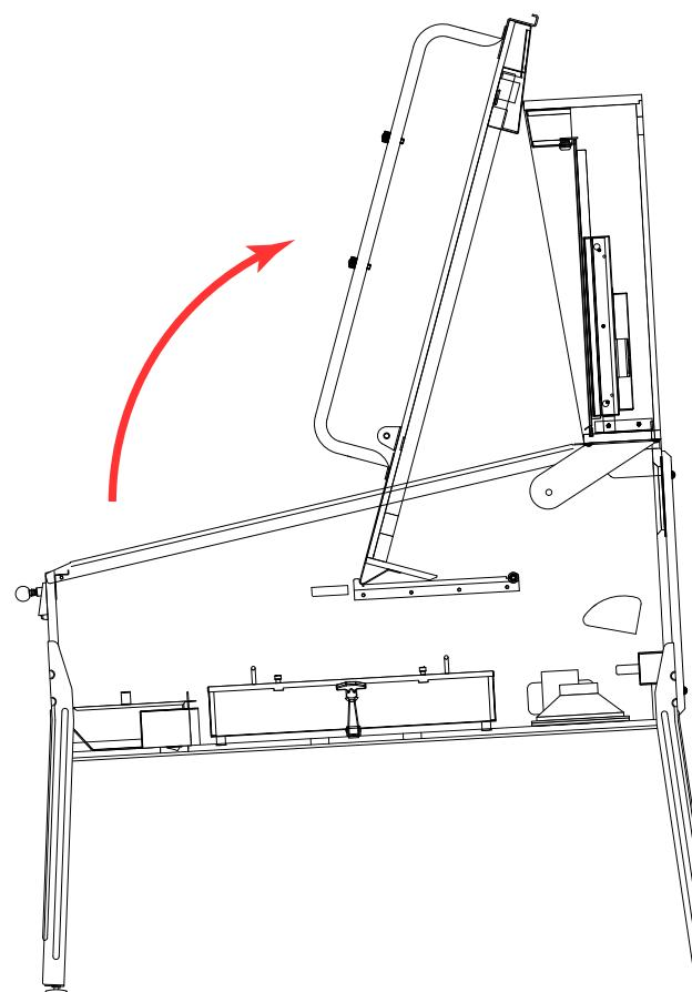
Figure A15. Moving the playfield to position 4.
