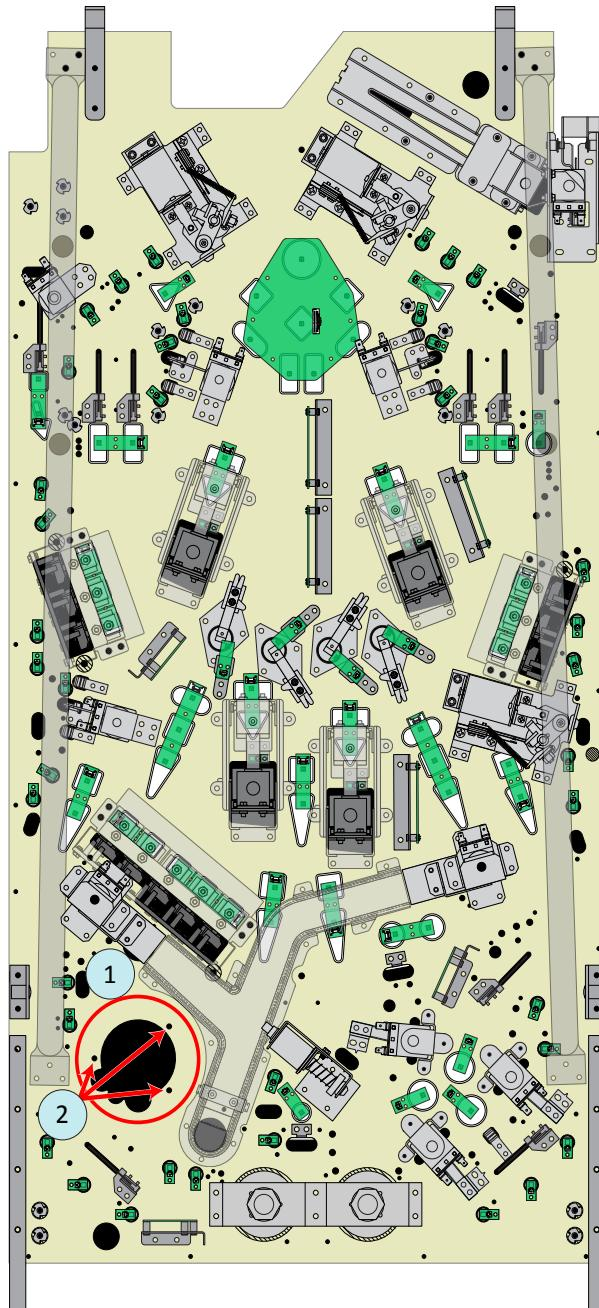
Figure E1. Playfield underside - Smaug Assembly location.
