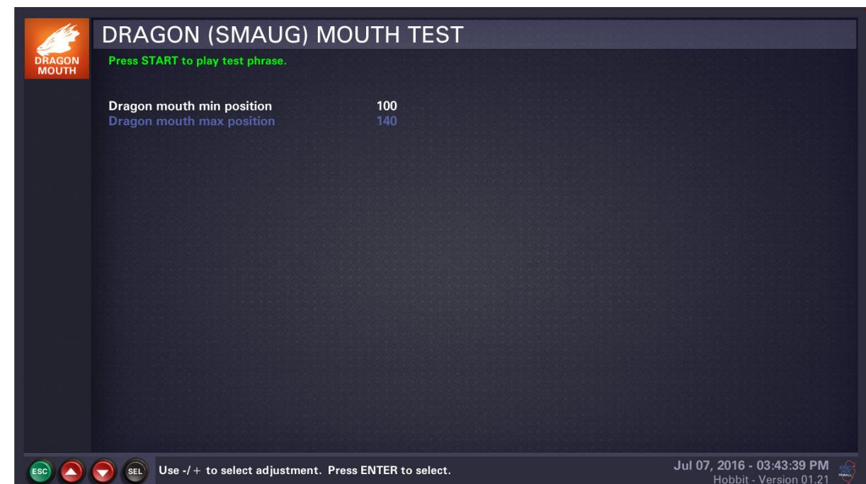
Figure E6. Smaug Mouth Test diagnostics screen.
