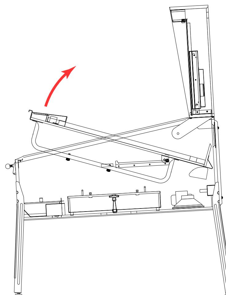
Figure A12. Swing the playfield upward.
