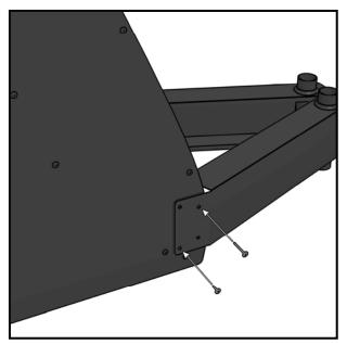
Tighten both screws with a 4mm Hex Wrench. Be sure the screws are tightened securely, but do not over tighten.
