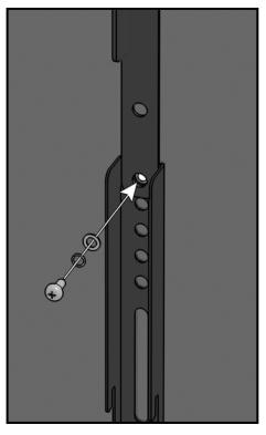
Once positioned, attach the vertical brackets with the appropriate combination of screws and washers designed for your screen. Tighten screws so the brackets are firmly secured, but take care not to overtighten or stress your hardware.
