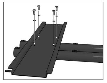
NOTE: If you wish to mount your monitor lower to the ground, attach the monitor plate to the lower sets of screw holes on the poles.
