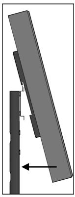
Use an assistant to carefully lift the HDTV and position it in front of the Monitor Bracket. Hook the two Vertical Brackets onto the top bar of the Horizontal Monitor Plate, then slowly swing the screen down and into place against the lower bar of the plate.
