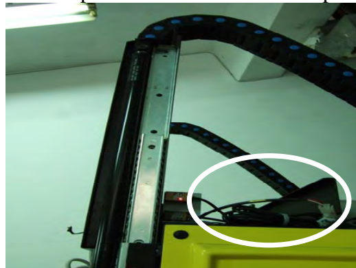
(b) Check the connector (UD_MOTOR) on the top side of cockpit. The wire should not be pulled out.
