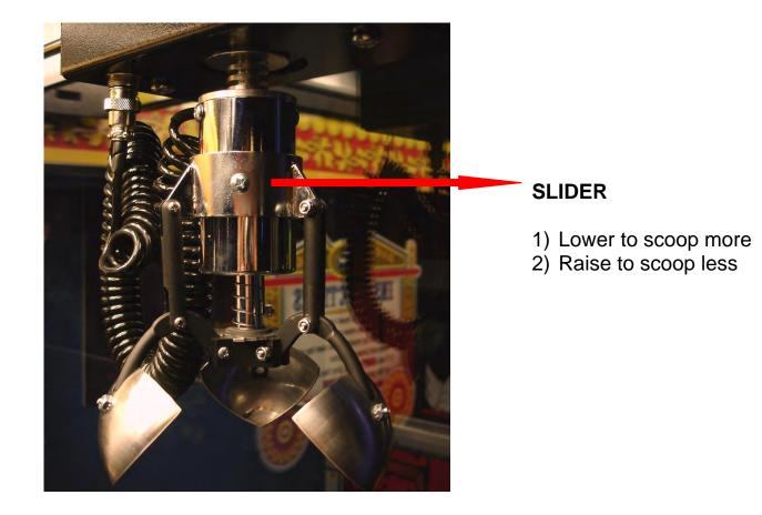
The slider is the part of the claw assembly that affixes the claw fingers to the core (solenoid housing). There are 3 Philips head screws that allow an operator to raise or lower the slider in order to achieve the most effective "scoop" action for a mix of candy.
