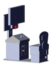
Place the upper monitor assembly down on it's face and remove the four nuts and bolts. It is recommended to use two people to lift the monitor out of the assembly.
