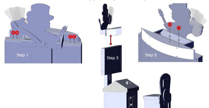
Now remove the four side mounting bolts (two on each side) and the two back bolts.
