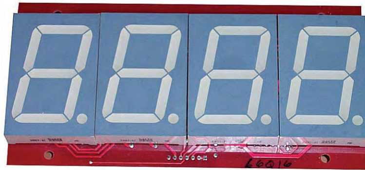
CC2033X— Jackpot Display PCB (front)
