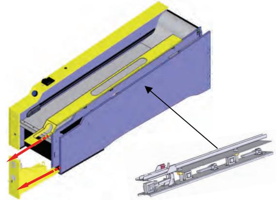
Slide both the cash box and ball release cover out and out of the way. Remove the foam packing material located on top and underneath the ball release assembly. Replace the cover and coin door.
