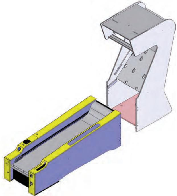
6. Open the ticket door and slide the top left cover back and then off to access the wire harnesses. Connect the six wire harnesses. If installing more than one game see "Link Install Instructions" before continuing.
