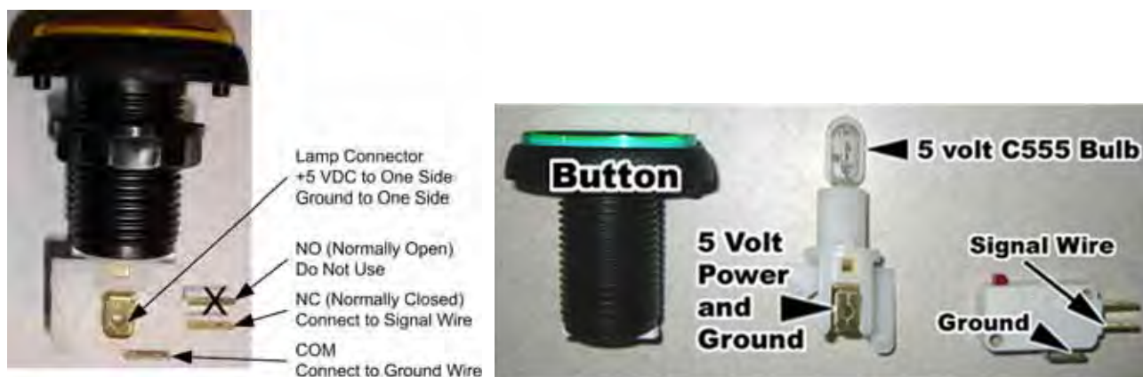
Figure 22. Replacing Button Components
