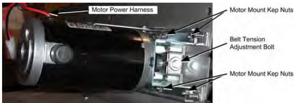
Figure 20. Servicing the Steering Motor
