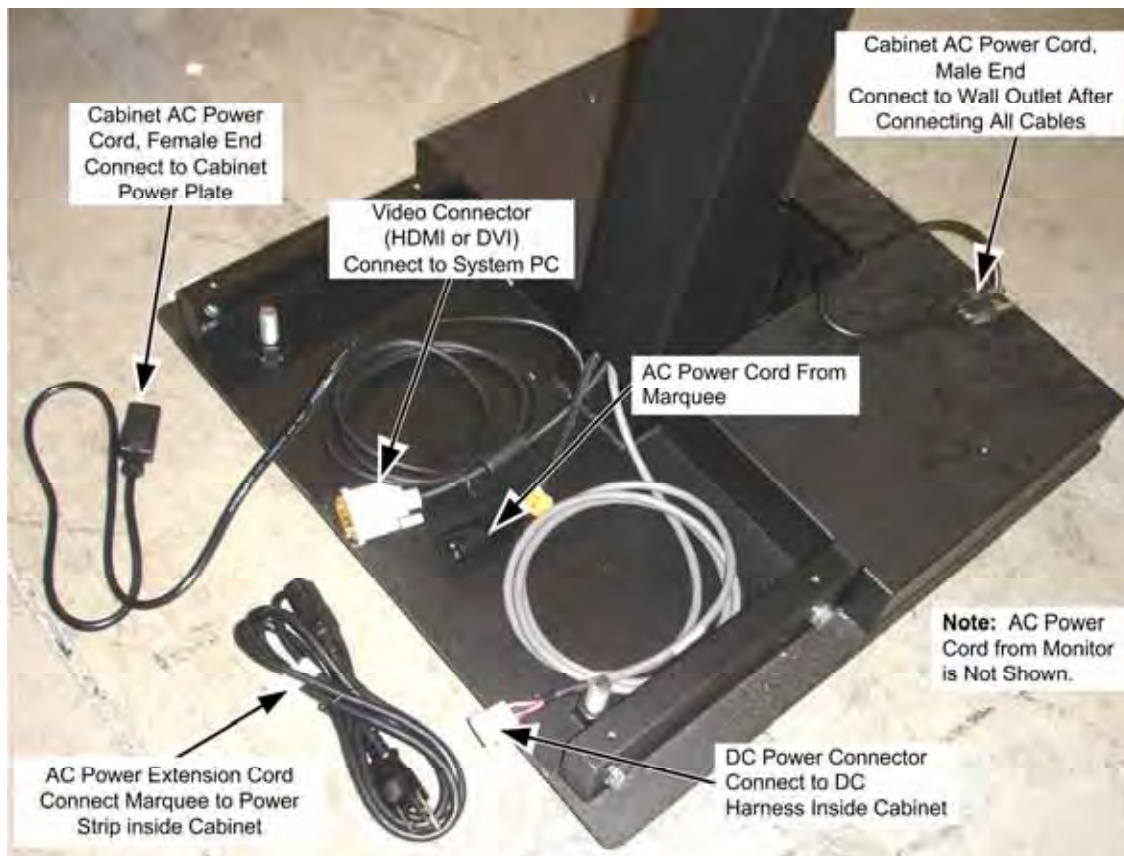
Figure 4. Cables in Display Stand Base
