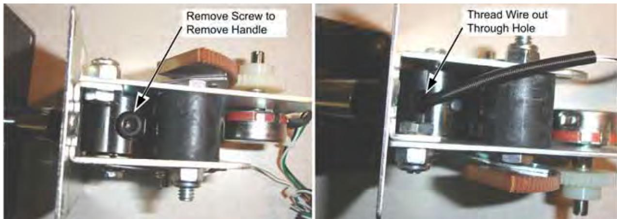
Figure 17. Replacing the Throttle Handle
