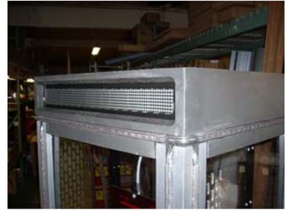
5. With an assistant, lift the top trim section onto the lid of the machine. Face the moving message sign towards the front (above the timer display). Make sure that the rope lighting ends from the corner sections are inside the top trim and not being pinched. Allow the section to rest on the top of the corner trim pieces (Fig F).
