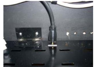
7. While still using a step ladder, unlock and remove the access lid on the top of the machine. Using (2) ½” X 10-32 screws and nuts supplied, secure the top trim section to the top of the machine by inserting a screw up through the top of the machine from inside the unit and tighten the nuts at the top (fig I).
