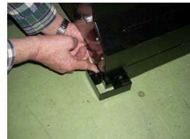
3. With an assistant, stand the complete unit upright. Locate and install the 4 corner trim cups to the bottom of the base using the (4) 10-24 X 1" carriage bolts and nuts provided. Fasten a cup to each lower corner of the base by inserting the bolts through the cup and the 1/4" unused round holes in the base from step #1. Tighten the nuts securely under the base (fig. D).
