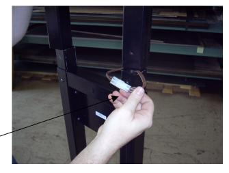
14. Once the rope light cord has been connected and tucked into the tube, slide the upper mast down onto the lower mast splice tubes and attach with (2) ½-20 x ½"screws. You may have to loosen the screws in the lower mast for alignment. Make sure the clicker shaft at the top is pointing forward (away from you) as well as the wheel shaft. You may now fully tighten all upper mast screws.
