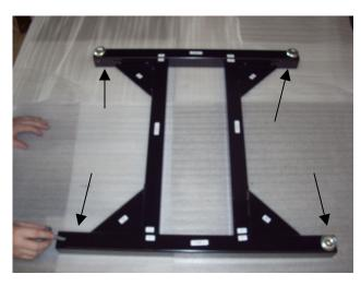
4. Locate the ¼" tapped holes at the inside ends of tubes 1 and 2. Slide a wheel lockwasher over each wheel assembly bolt and attach the wheel assemblies to the base. Both wheels must be on the left or right side (A and C end or B and D end). Do not over-tighten.
