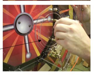
24. Locate the 24 wheel pins and nuts. Attach pins to the wheel by inserting one pin at a time through the outer holes in the wheel and securing with a nut on the rear side. This will require a screwdriver and 3/8" wrench. Do not over tighten.
