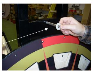
18. Slide the 48" wheel on to the wheel shaft with the bearing hub towards the rear. This may require an assistant.
