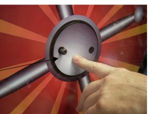
23. Reattach the locking door to the front of the tumbler assembly and lock in place.
