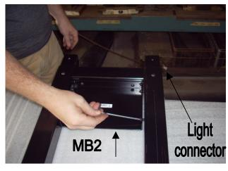
9. Stand the lower mast assembly upright with the wheel shaft at the top and facing forward. Attach the lower mast to the 2 braces (MB) on the base assembly with (4) ½-20 x ½" screws. You may now fully tighten all (12) screws used in the assembly process to this point.
