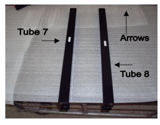
12. Locate and attach upper mast brace (MB3) using (4)  $^{1}4$ -20 x  $^{1}2$ " screws to the inside of tubes 7 & 8. Make sure the decal is face up and the arrows on the brace are pointing the same direction as the arrows on tubes 7 & 8. The clicker shaft will be pointing downward and it will make attaching this part easier to allow the shaft to hang over the assembly bench as well. Do not fully tighten.
