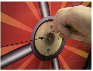
22. Attach the tumbler center cap over the end of the shaft with  $(2) \frac{1}{4}$ -20 x 1" screws.
