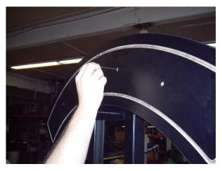
17. Locate (1) wheel shim washer and slide it on to the wheel shaft at the center of the lower mast.
