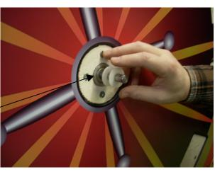
20. Locate the tumbler assembly and remove the locking door. Slide the tumbler assembly on the wheel shaft. The "c" clip groove should be visible on the end of the shaft. If it is not visible, you may need to remove one washer from behind the tumbler assembly.
