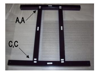
2. Attach 4 base braces (BB) to each intersection of tubes 1 thru 4 with (16) ½- 20 x 1/2 " screws. Make sure the labels on the braces face upward. Do not tighten completely until all screws have been started. Make sure not to over-tighten!
