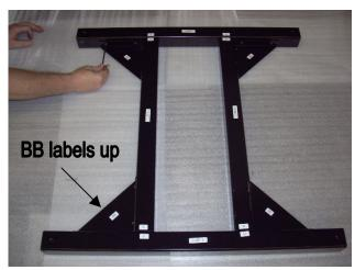
3. Insert (4) base levelers into the 3/8" tapped holes at each end of tubes 1 and 2. Screw them down completely.
