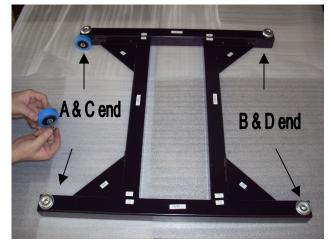
5. Flip the base assembly over. Locate the (4) ¼" tapped holes on the top of the center tubes. Attach the (2) mast braces (MB) with (4) ¼-20 x ½" screws. Position the braces so that the labels face each other (inward) and the vertical legs of the braces are towards the center of the base. Do not tighten completely until later. This portion of the assembly can now be set aside.
