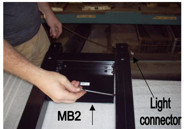
9. Stand the lower mast assembly upright with the wheel shaft at the top and facing forward. Attach the lower mast to the 2 braces (MB) on the base assembly with (4) ¼-20 x ½” screws. You may now fully tighten all (12) screws used in the assembly process to this point.
