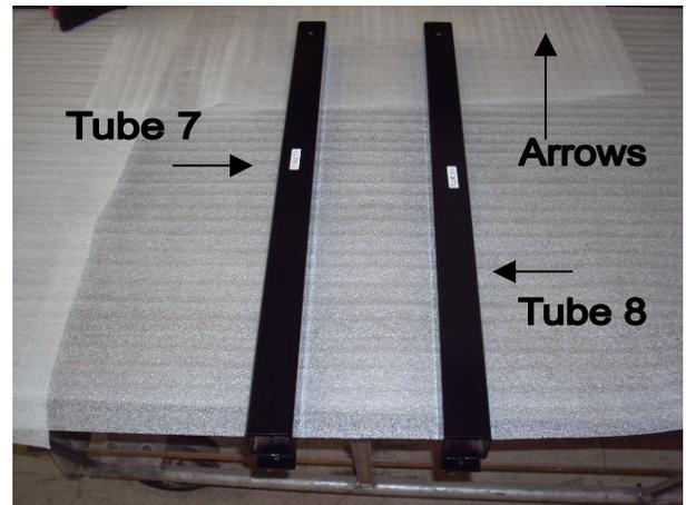
12. Locate and attach upper mast brace (MB3) using (4) ¼-20 x ½” screws to the inside of tubes 7 & 8. Make sure the decal is face up and the arrows on the brace are pointing the same direction as the arrows on tubes 7 & 8. The clicker shaft will be pointing downward and it will make attaching this part easier to allow the shaft to hang over the assembly bench as well. Do not fully tighten.
