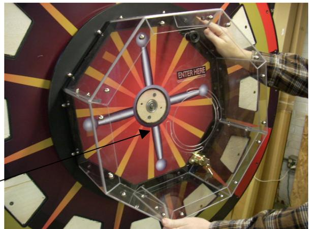
21. Attach the “c” clip to the groove on the shaft to secure the tumbler and wheel in place.
