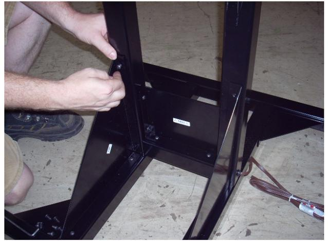
10. Your assembly should now resemble the photo to the right. Make sure that the wheel shaft is facing forward and the mast braces are at the rear.
