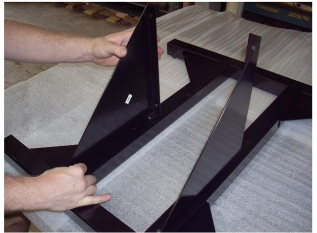
6. Assemble the lower mast by placing tube #5 and #6 on a flat surface with tube #5 on the left and tube #6 on the right. Make sure the decals are facing up and the arrows are pointing upward as well (away from you). These tubes will also have splice tubes protruding from the top end as well.
