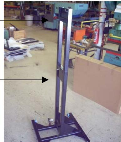
16. Locate and attach the wood header to the "u" bracket at the top of the upper mast with (2) 10-32 x 1" screws. This step may require use of a step ladder. Use the two thru holes toward the center of the header. Make sure the rope light is facing forward and the cord does not get pinched on the back side. Fully tighten.
