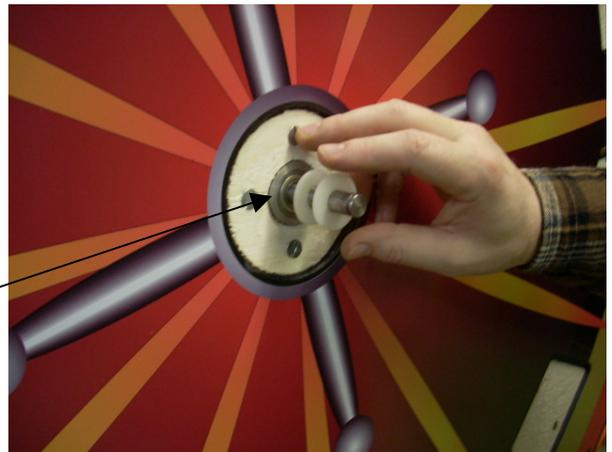
20. Locate the tumbler assembly and remove the locking door. Slide the tumbler assembly on the wheel shaft. The "c" clip groove should be visible on the end of the shaft. If it is not visible, you may need to remove one washer from behind the tumbler assembly.
