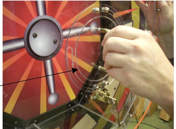
24. Locate the 24 wheel pins and nuts. Attach pins to the wheel by inserting one pin at a time through the outer holes in the wheel and securing with a nut on the rear side. This will require a screwdriver and 3/8" wrench. Do not over tighten.
