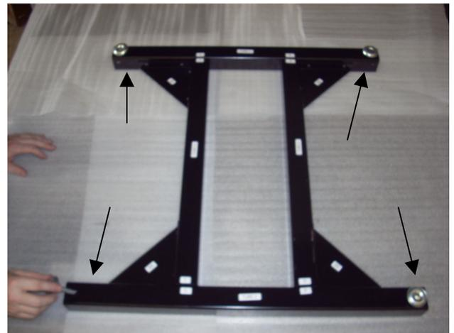
4. Locate the ¼” tapped holes at the inside ends of tubes 1 and 2. Slide a wheel lockwasher over each wheel assembly bolt and attach the wheel assemblies to the base. Both wheels must be on the left or right side (A and C end or B and D end). Do not over-tighten.
