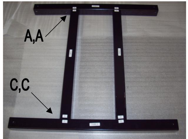
2. Attach 4 base braces (BB) to each intersection of tubes 1 thru 4 with (16) ¼- 20 x 1/2 “ screws. Make sure the labels on the braces face upward. Do not tighten completely until all screws have been started. Make sure not to over-tighten!
