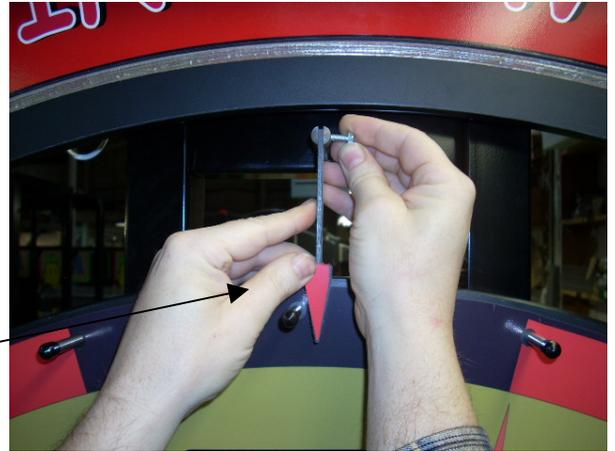
27. Attach the printed footer panel to the front of the lower frame legs using (4) 10-32 x 1/2" screws.
