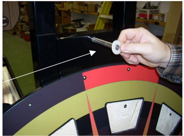
18. Slide the 48" wheel on to the wheel shaft with the bearing hub towards the rear. This may require an assistant.
