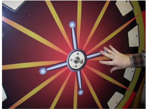
19. Locate (3) wheel shim washers and slide them on the wheel shaft.
