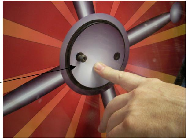
23. Reattach the locking door to the front of the tumbler assembly and lock in place.
