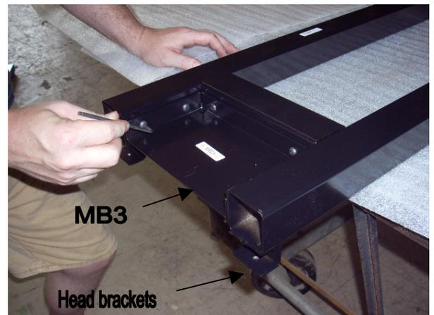
13. Lift the upper mast assembly and prepare to slide it onto the splice tubes of the lower mast assembly. Make sure the clicker shaft is at the top and pointing forward (same direction as wheel shaft on lower mast). Before attaching to the lower mast, connect the two light cord leads together and tuck the excess cord down into the tube. This may require an assistant.
