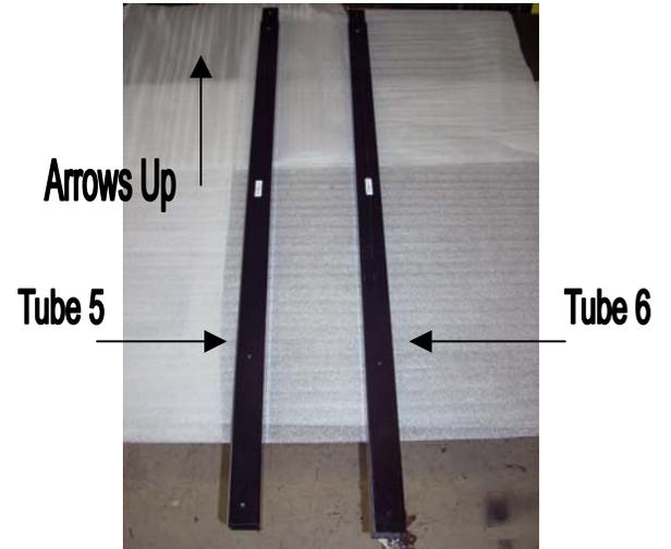
7. Locate the bottom lower mast brace (MB1). Making sure the decal is facing up and the arrow on the decal is pointing the same direction as the arrows on tubes 5 & 6, attach the brace to the inside lower end of tubes 5 & 6 with (4) ¼-20 x ½” screws. Do not fully tighten.
