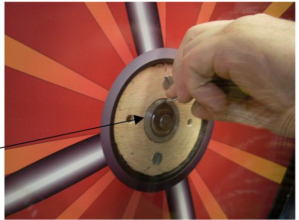
22. Attach the tumbler center cap over the end of the shaft with (2) 1/4-20 x 1" screws.
