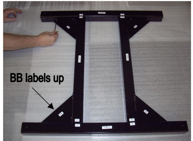
3. Insert (4) base levelers into the 3/8” tapped holes at each end of tubes 1 and 2. Screw them down completely.
