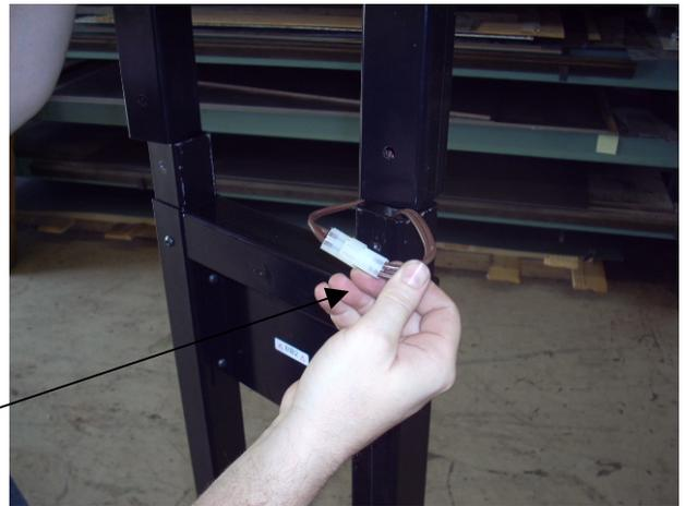
14. Once the rope light cord has been connected and tucked into the tube, slide the upper mast down onto the lower mast splice tubes and attach with (2) 1/4-20 x 1/2" screws. You may have to loosen the screws in the lower mast for alignment. Make sure the clicker shaft at the top is pointing forward (away from you) as well as the wheel shaft. You may now fully tighten all upper mast screws.
