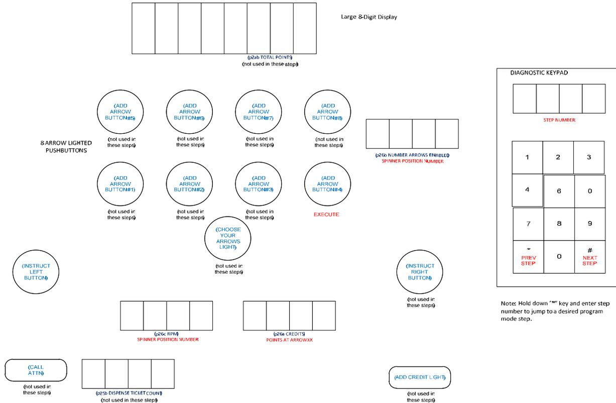
Note: Hold down "\*" key and enter step number to jump to a desired program mode step.
