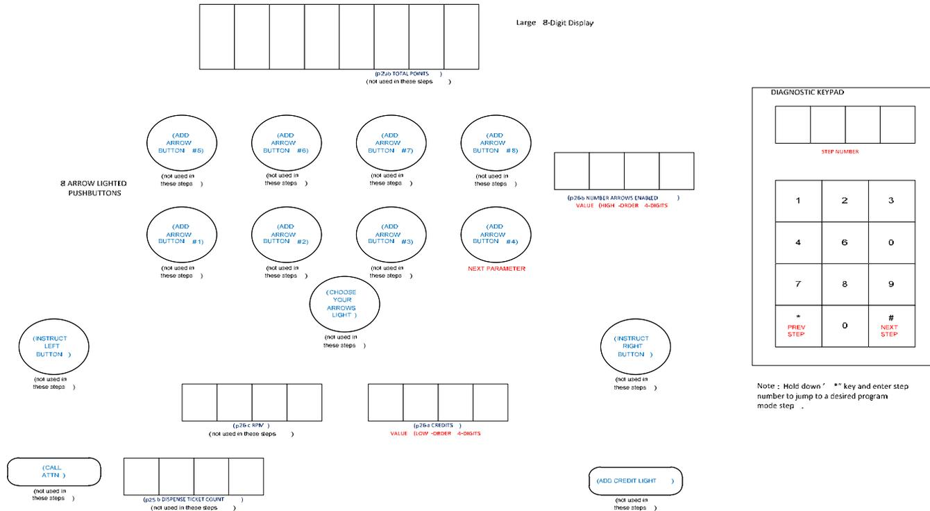
To increase the **STEP NUMBER** use the Numeric Keypad and press the “\*”, to decrease the **STEP NUMBER** press the “#” symbol. To Go to **STEPS** directly Hold down the “\*” key while entering the **STEP NUMBER** in the keypad. To View Statistics Press the **#4 BUTTONS** to cycle through each Statistic.
