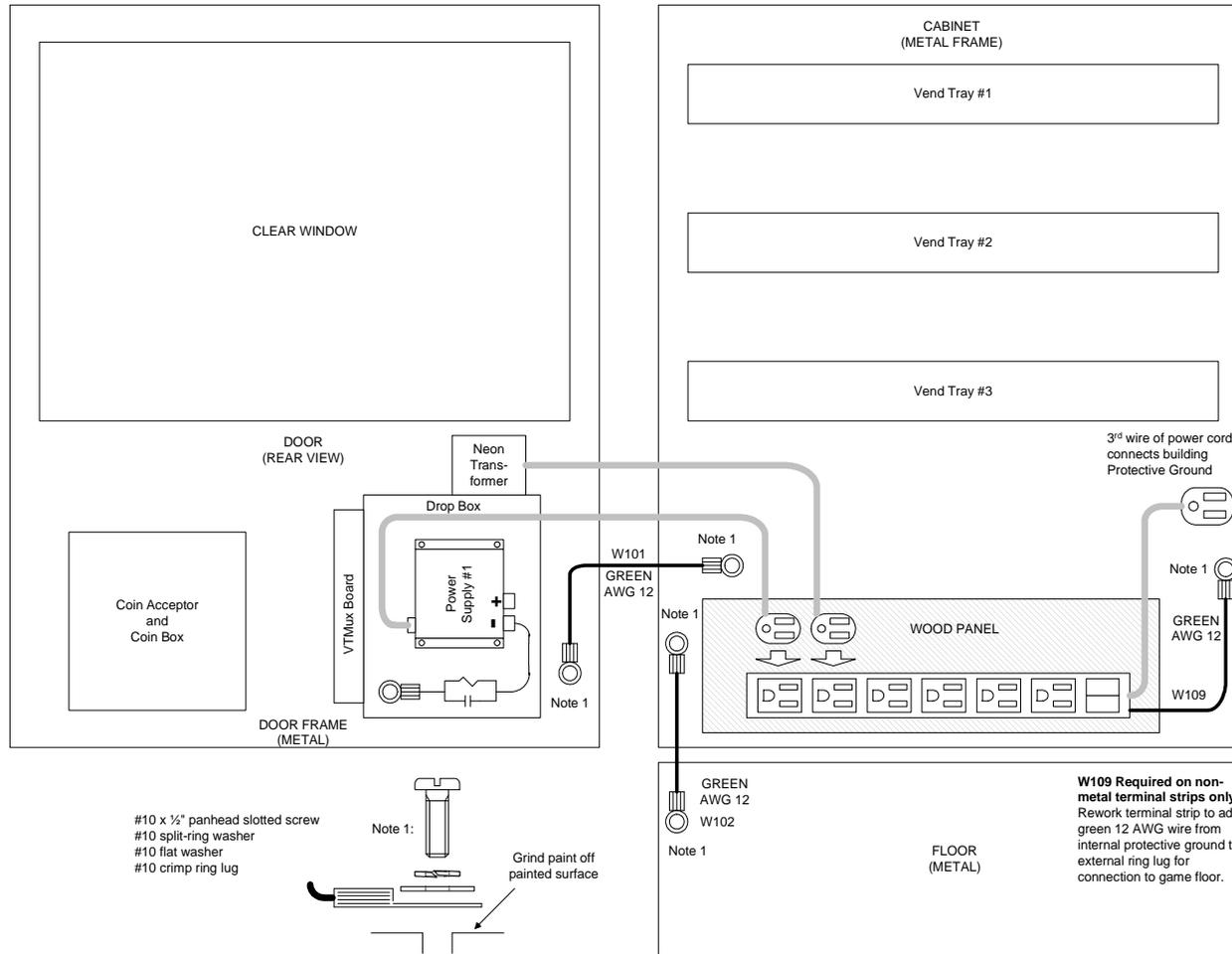
**FIGURE 30 - PROTECTIVE GROUND WIRING**
