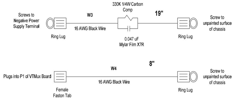
Figure 19 Topper Lights Wiring
