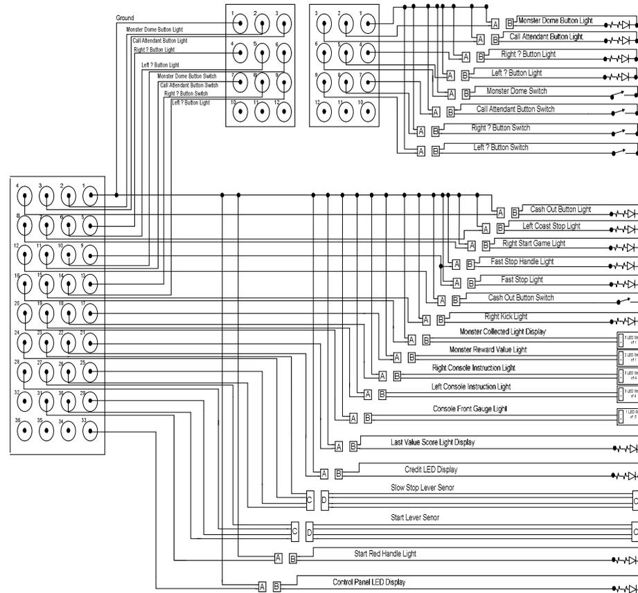
**FIGURE 5 CONNECTIONS TO THE CONTROL PANEL**
