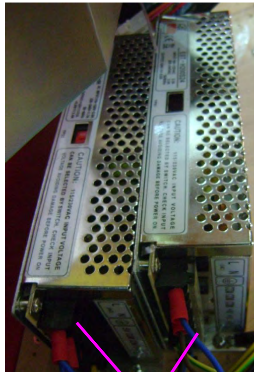
Power Supply REA-E-16 (12V + 5V) REA-E-17 (24V)
