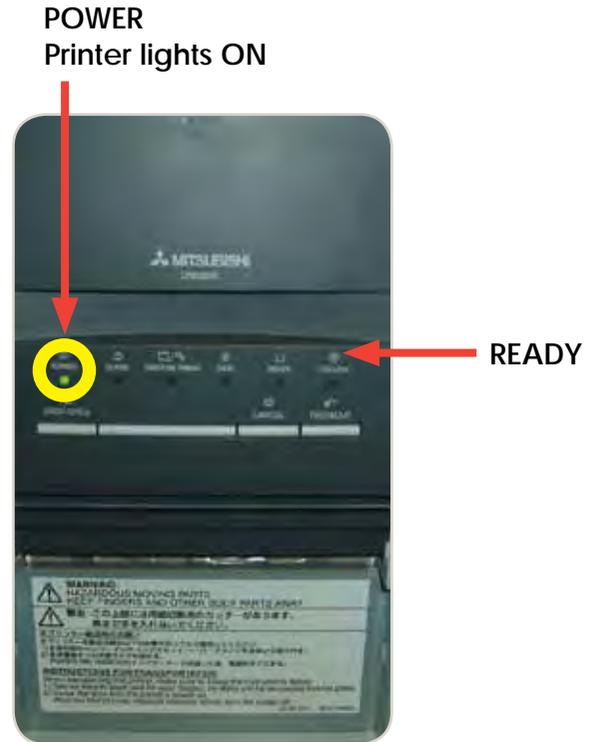
2- Check the Printer Connections. Power and USB, just 2 wires.
