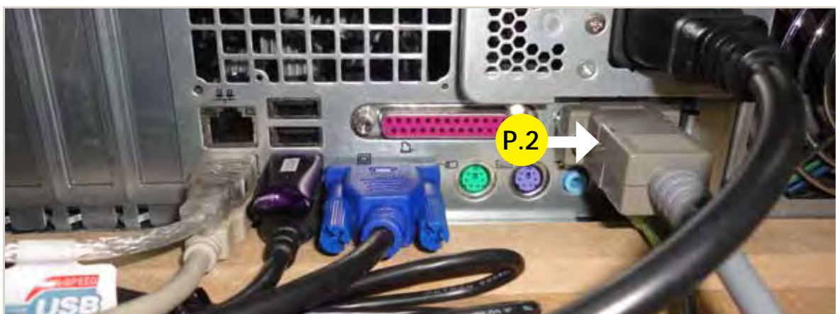
P.2 Serial Cable From Control Board to PC. (56 cm - Inch 22,04)
