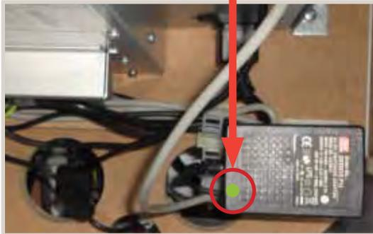
If the power card is properly plugged then the LED is blue.
