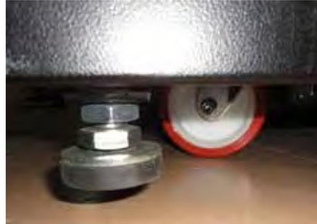
Adjust the height of the four metal legs once the final location for the booth has been established. The metal legs are underneath the cabin next to the wheels.
