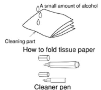
When lines appear on the printed images, clean the thermal head.
