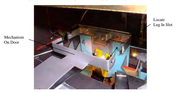
Moving Coin Entry Mechanism
