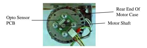
Opto Sensor PCB Mounted To Motor
