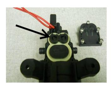
3. Carefully remove both diaphragms and clean with light soap and water. Re-install and test.
