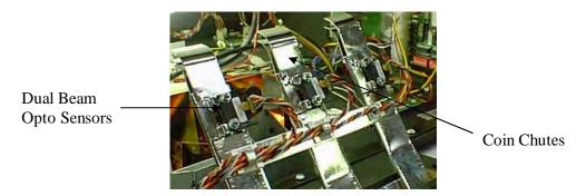
Coins enter via one of three coin chutes and pass through a dual beam coin sensor. These are connected to an interface board, which generates a coin-in signal. This signal is directed to the section logic board, which in turn activates the player section and increments the coin-in counter.
