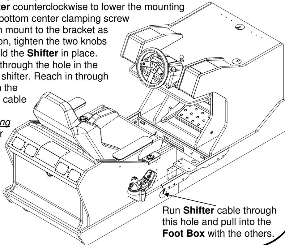
Run **Shifter** cable through this hole and pull into the **Foot Box** with the others.
