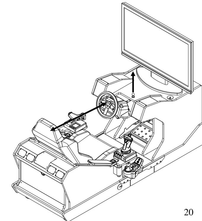
To move the steering wheel forward or back, pull up on the release knob and move the shelf in the direction you need.
