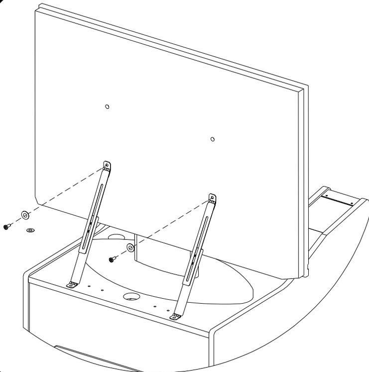
Find the bag labeled TV Bracket Hardware, which contains four different types of screws and some washers. The three sets that look similar are different sizes used to connect wall-mounting brackets to different televisions. Usually, the larger the television, the larger the screw used. Find the set of screws that fit the mounting holes on the back of your television.
