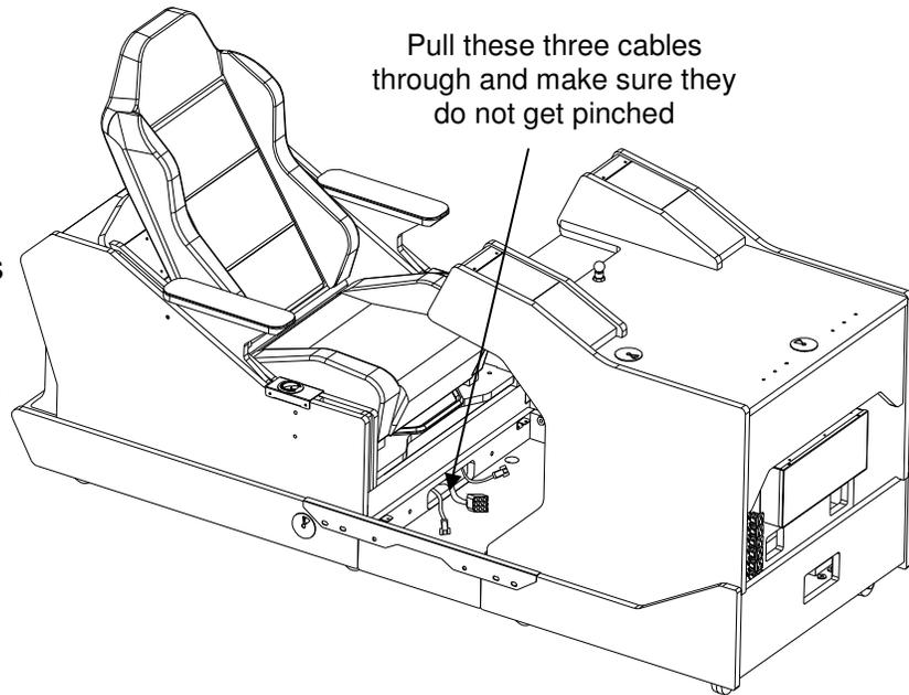
Use the eight remaining bolts and washers in the bag labeled Connector Bracket Hardware to connect the **Foot Box** to the other two cabinets through the **Connector Brackets**.
