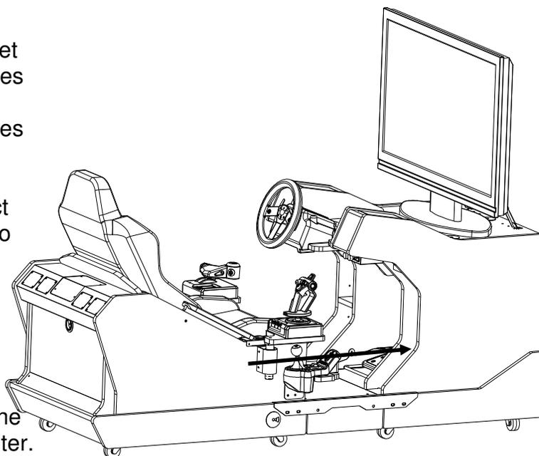
You can also install your computer in the rear cabinet. In order to do this, you will need some longer cables that are not included. Run the computer cables through the cabinet under the seat. These cables can be found at an electronics store or PI Manufacturing's website, [www.PIMFG.com](http://www.PIMFG.com). The part numbers for these cables on PI Manufacturing's site are:
