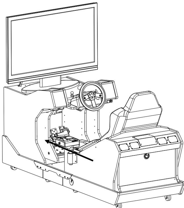
Slide your Playstation into the cabinet on the left side. Running the cables through the back of the cabinet, connect the HDMI cable to the Playstation and HDMI port on the television. Connect the power cord to the Playstation and power strip. Connect the USB cable labeled **PS3** to the front USB port on the Playstation.
