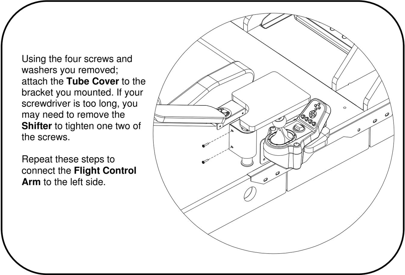
Using the four screws and washers you removed; attach the **Tube Cover** to the bracket you mounted. If your screwdriver is too long, you may need to remove the **Shifter** to tighten one two of the screws.
