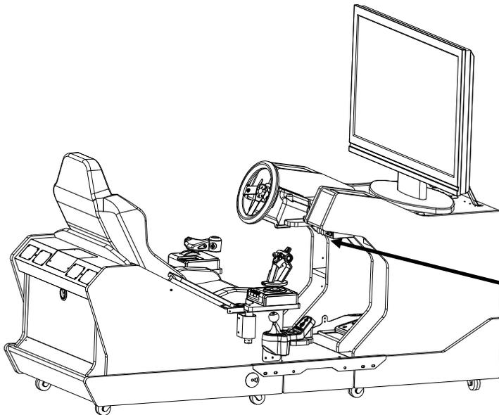
The main power switch, volume control knob and bass shaker knob are located below the right speaker
