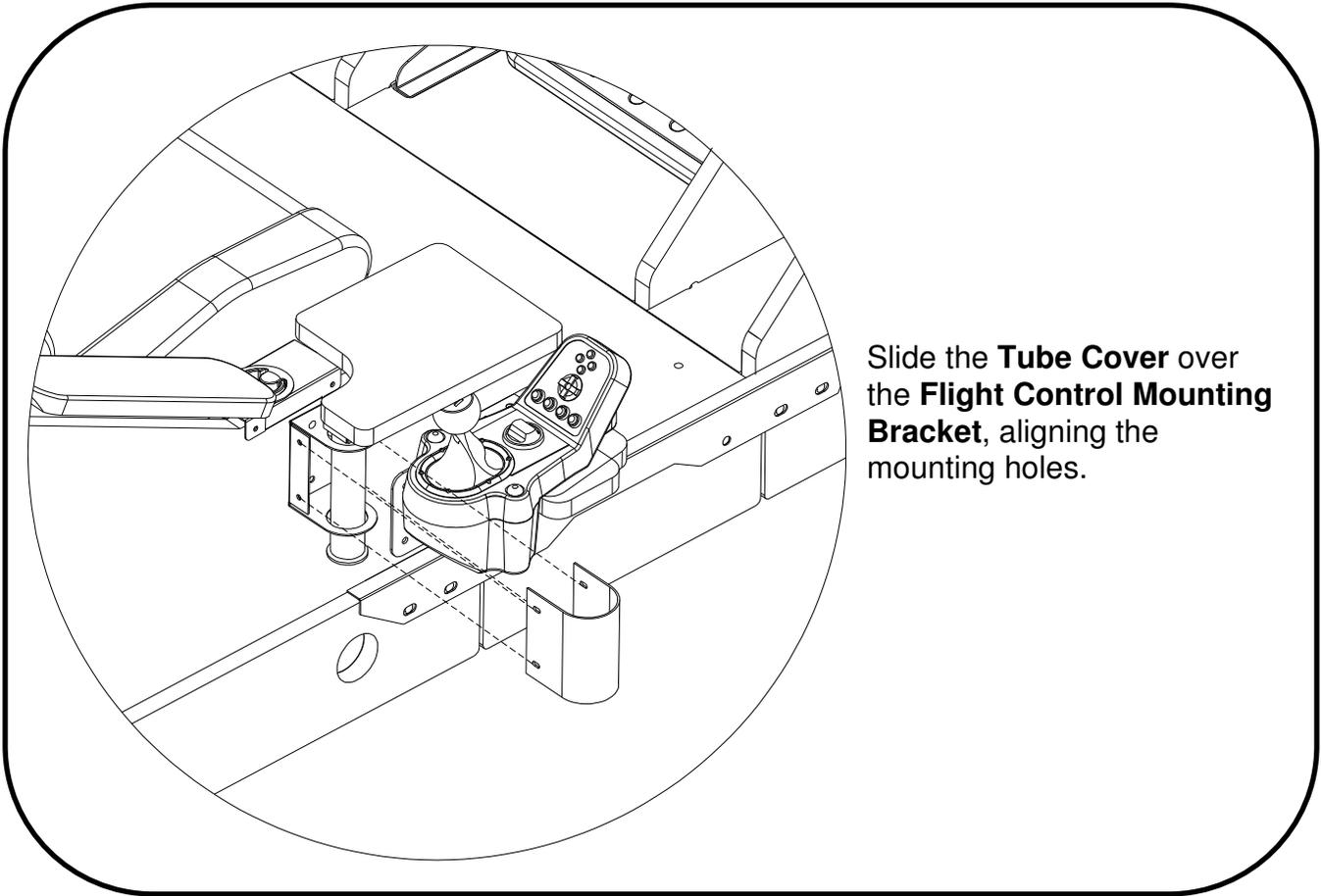
Slide the **Tube Cover** over the **Flight Control Mounting Bracket**, aligning the mounting holes.
