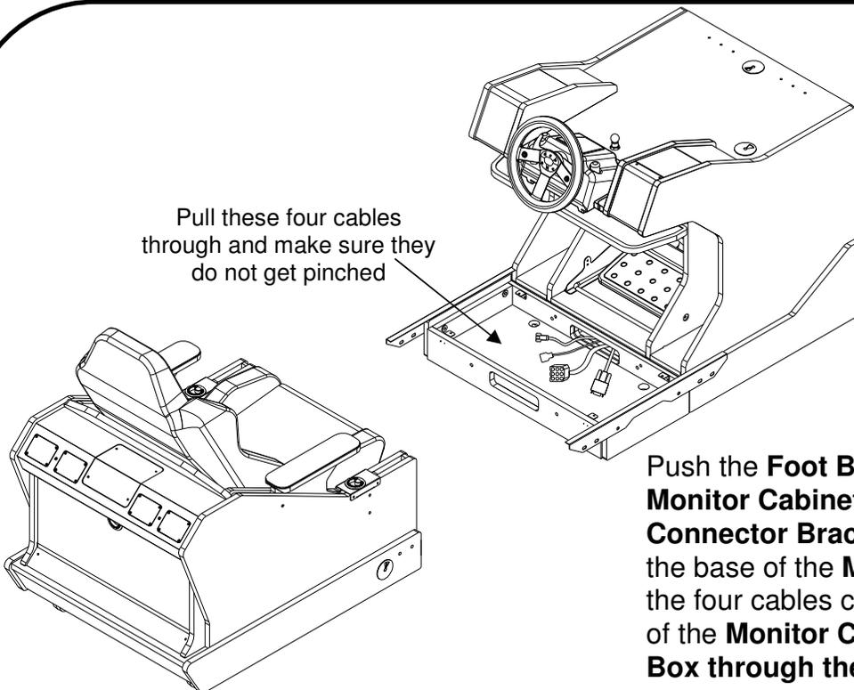
Push the **Foot Box** up against the **Monitor Cabinet** so the **Cabinet Connector Brackets** are resting on the base of the **Monitor Cabinet**. Pull the four cables coming from the bottom of the **Monitor Cabinet** into the **Foot Box** through the rectangular hole.
