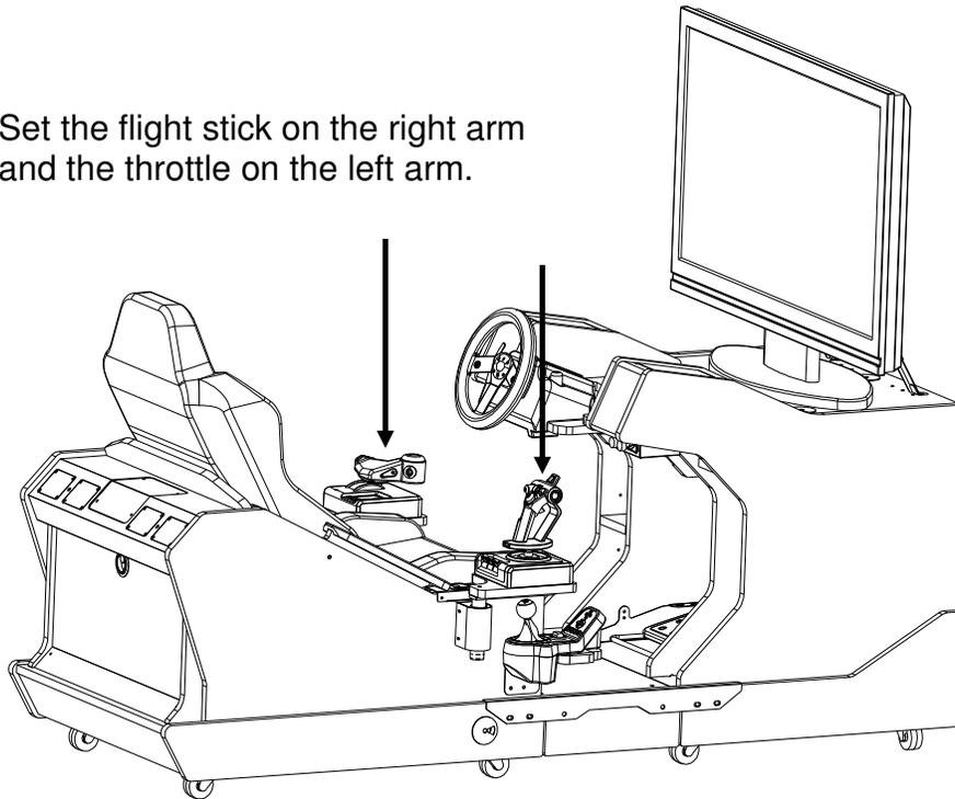
Secure the flight controls to the mounting arms with the screws in the bag labeled Saitek Control Hardware. Each piece is held in place with two screws, circled here.
