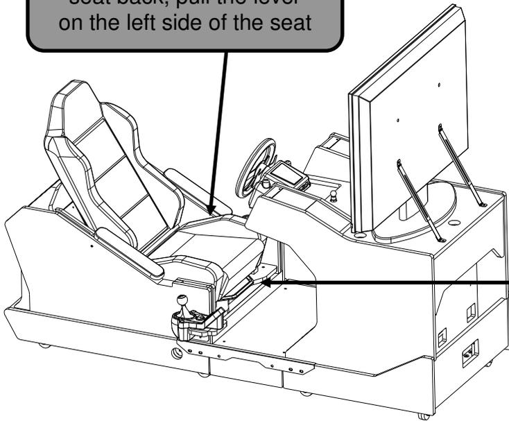
To move the seat forward or back, lift up on the release bar under the front of the seat
