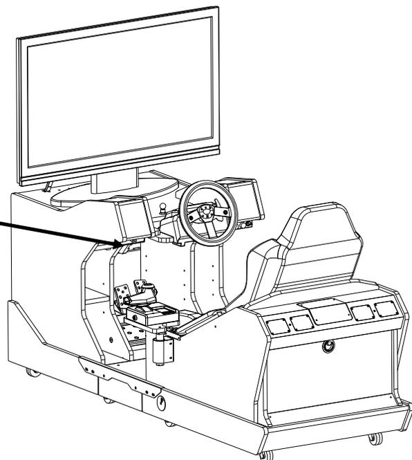
The electronics case is located in the back of the **Monitor Cabinet**. This contains the power supply and amp for the speaker system. The 3.5mm audio jack is on the top right side of the electronics case.
