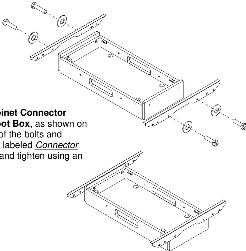
Attach the two **Cabinet Connector Brackets** to the **Foot Box**, as shown on the right. Use four of the bolts and washers in the bag labeled Connector Bracket Hardware and tighten using an Allen wrench.
