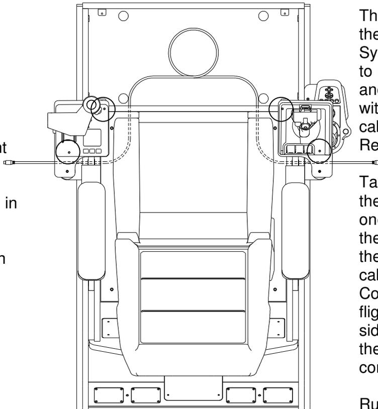
The cable that comes with the Saitek X52 Flight System is slightly too short to run through the cabinet and connect the flight stick with the throttle, so a longer cable is included with Redline GT.
