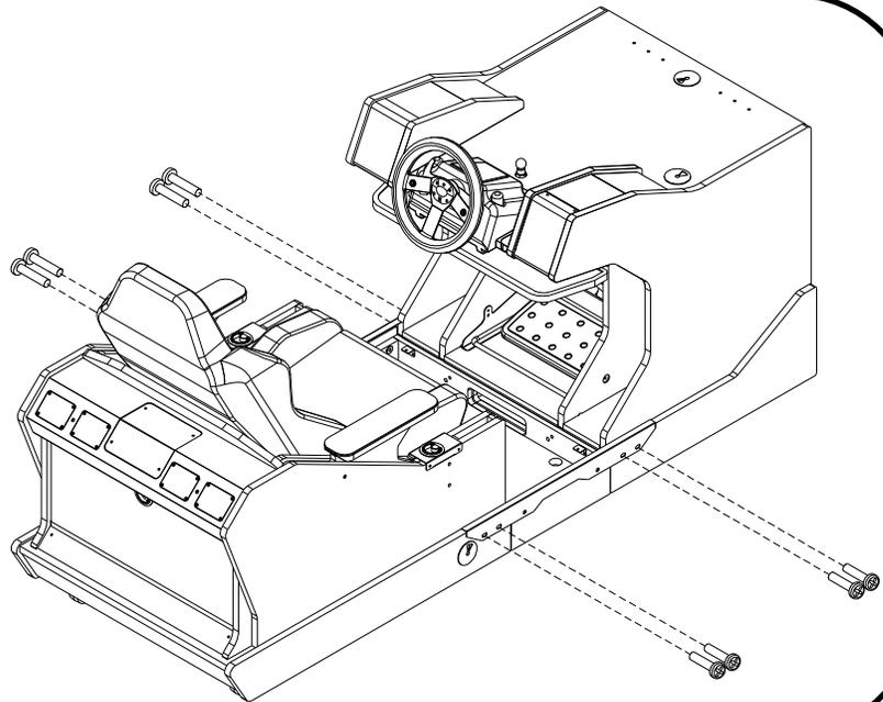
Use the four bolts and washers in the bag labeled Foot Box Connect Hardware to connect the **Foot Box** to the **Monitor Cabinet** and **Seat Cabinet** as shown to the left. Tighten the bolts with a 7/16" wrench. Note that this image does not show the **Monitor Cabinet** or **Seat Cabinet** so that you can easily see where the bolts attach. After these bolts are tightened, tighten the outside bolts with an Allen wrench.
