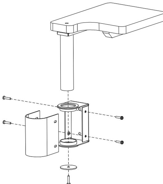
Remove the two screws on the side of the **Seat Cabinet** just below the armrest release. These will be used to connect the **Flight Control Arm** to your cabinet. Align the **Flight Control Arm Mounting Bracket** with the mounting holes, and attach the bracket with the screws you just removed.
