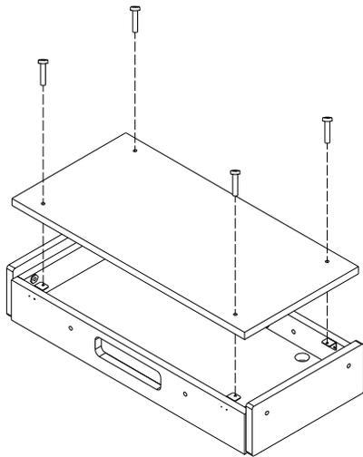
Start by removing the lid of the **Foot Box**. Remove the four Phillips head screws to free the lid, and it will pull straight up. Do not close the **Foot Box** until you have finished setting up and connected all of the cables.
