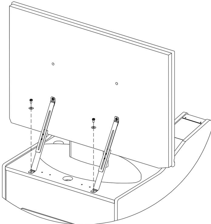
When you have adjusted the bracket to the correct length and aligned it with the pilot hole in the cabinet, use the two longest screws and two washers in the TV Bracket Hardware bag to connect the bracket to the cabinet. Tighten the screws that were loosened to adjust the length of the bracket.
