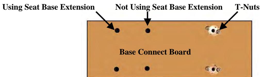
5. Facing the cabinet, fasten the board to the inside RIGHT of the CABINET with bolts until finger tight; some movement is required in the mounting boards to align holes with seat pedestal assembly. Use the appropriate mounting holes on the board and **make sure the screws holding the T-Nut in place are facing IN.**
