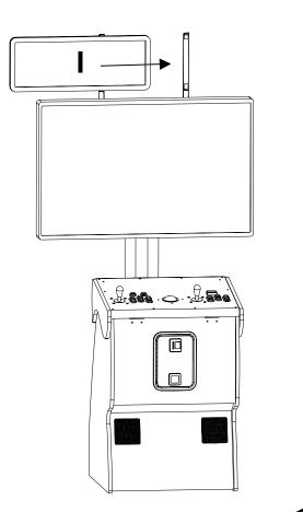
Run the 6' power cord through the hole in the back of part **B**. The 10' power cord from the television should already be coming out of this hole.
