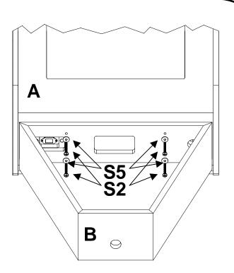
Adjust the leg levelers on part **B** so that it is level with the cabinet and the ground.
