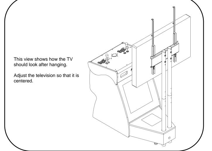
Tighten the screws at the bottom of part **G**, clamping the television to the mounting bracket.
