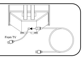
Reach inside part **B** and connect the power cord to the inlet plug, shown to the left. You now have two power cords coming out of the hole in part **B**. One powers the television, and the other powers the main cabinet.
