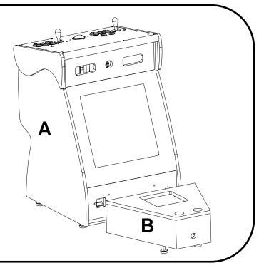
Align the square hole in part **B** with the wood block on the back of part **A**. Through the opening in part **B**, use 4 pieces of **S2** and **S5** to connect part **A** to part **B**. In the drawing on the right, the top of the box has been removed so you can more easily see where the bolts connect.
