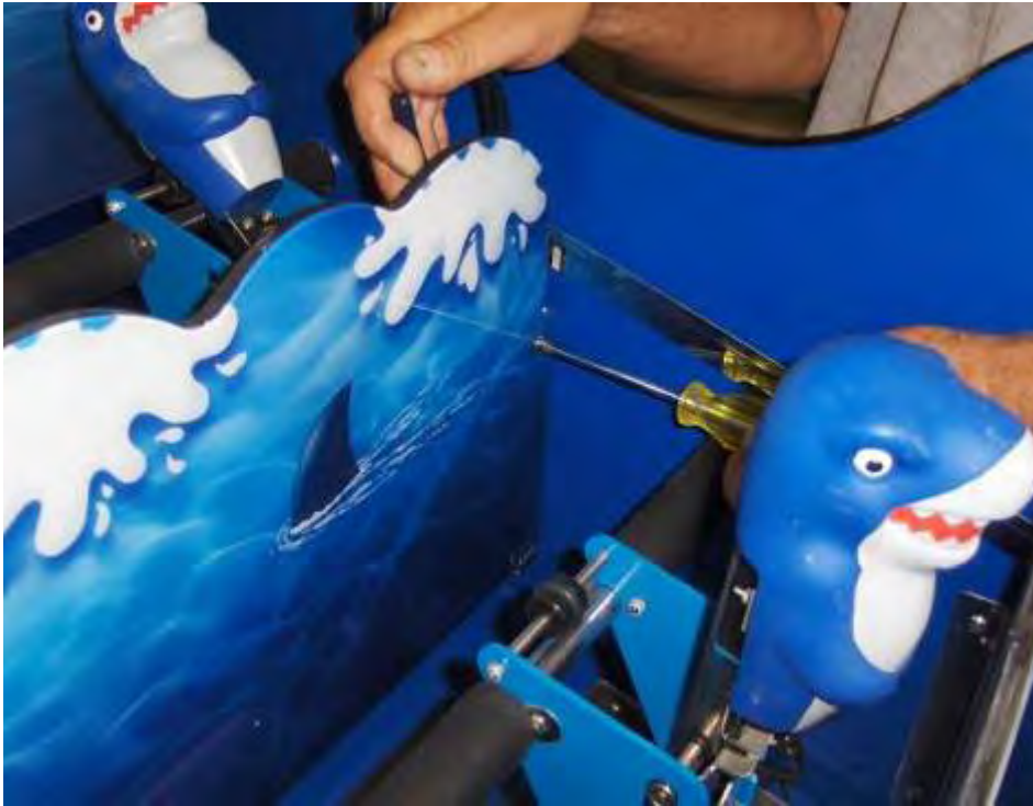
Fig. 4: Remove Wave by removing two screws and nuts
