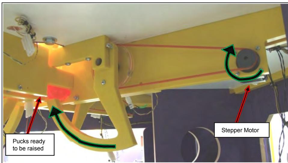
Figure 3, Puck Ramp Mechanism, Underneath Playfield Base.
