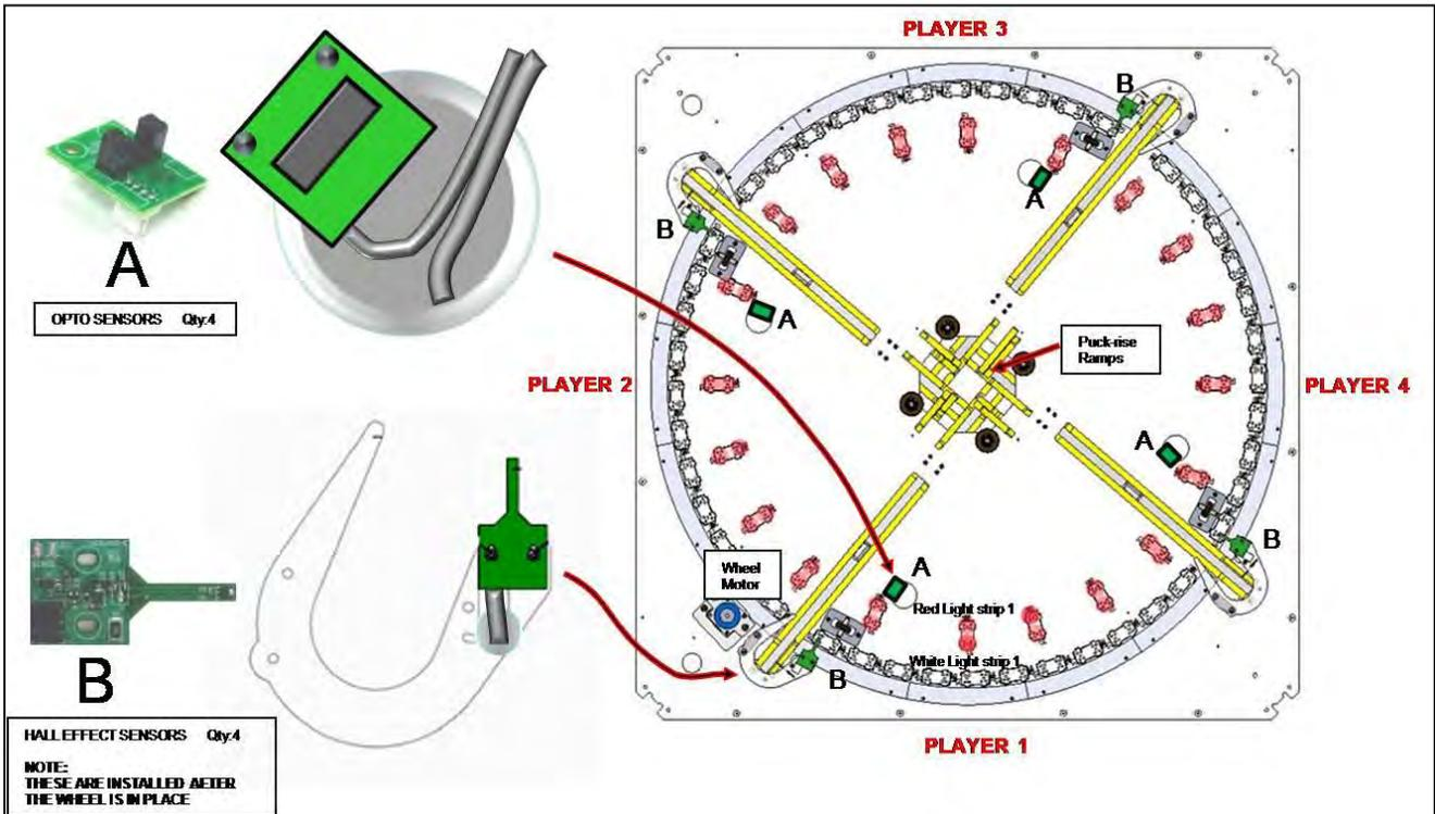
Figure 2, Game Sensors (Top View, wheel removed):
