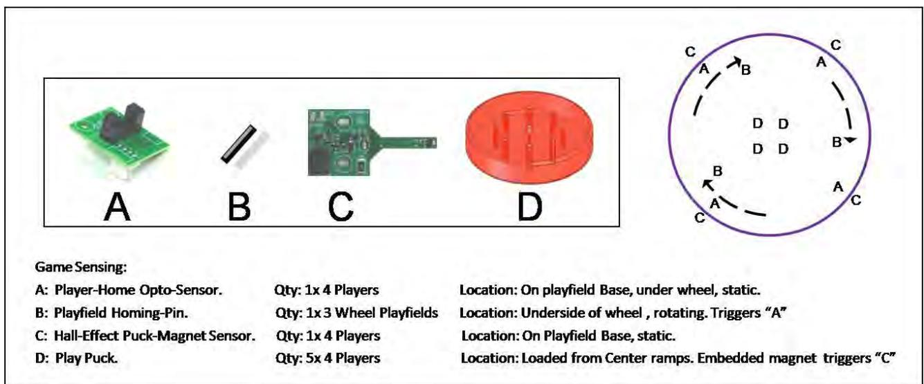
Figure 7. Sensing Components
