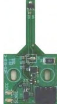
Detects the magnet embedded on the center of the Play-Puck, after It travels through the playfield.
