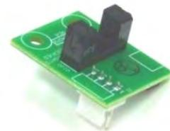
Detects the beginning of each Wheel playfield as it goes past the player side (the underside of the wheel has a pin for each playfield, which interrupts the Opto's IR beam). The signal is passed along as a low-level voltage transition (through a single wire, no 485) to the Quad-Stepper-2 Board, where the step position is annotated.
