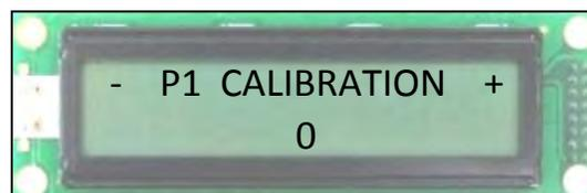
If there is still a small deviation, you can finely adjust the offset value on the LCD. Decrementing this value will turn the wheel counter-clockwise, while Incrementing it will turn it Clockwise. You have a range of about ¼” in both directions.
