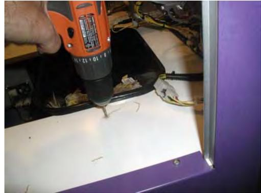
6. Mount the chute using the supplied screws.
