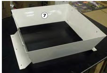
4. Place the new chute assembly⑦ on the ticket basket plate⑤ inside the machine. The chute should be approximately centered from left to right and from front to back. Use the ticket chute as a template to mark the ticket basket plate mount hole locations. Use the side doors for easier access.
