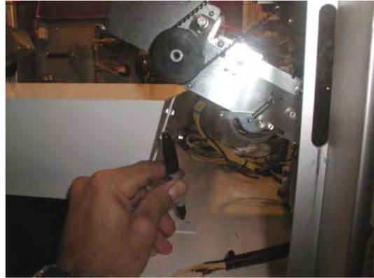
5. Using the marks, pre-drill mount screw holes using a 1/8" drill bit.
