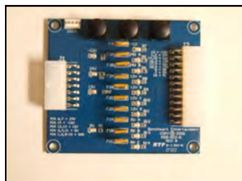
Power Distribution PCB
