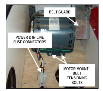
Figure 12 Conveyor Drive Belt Tensioning
