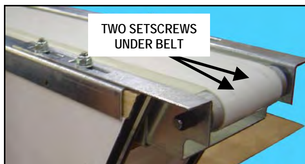
Figure 10 Belt Removal – Exit End
