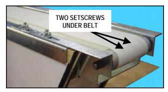
Figure 10 Belt Removal – Exit End
