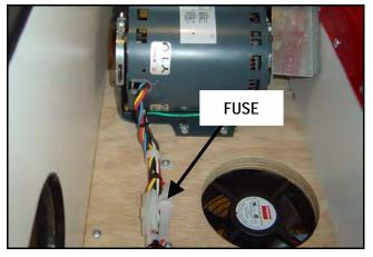
Figure 5 Conveyor Motor Fuse Use 5 amp Fast Burn fuse.
