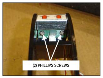
Figure 17 Coin Sensor Board
