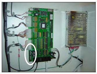
Figure 4 Dipswitch location on Gen 5 Main Board
