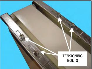
Figure 9 Conveyor Adjustment
