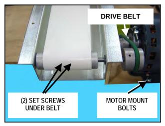
Figure 11 Belt Removal – Drive End
