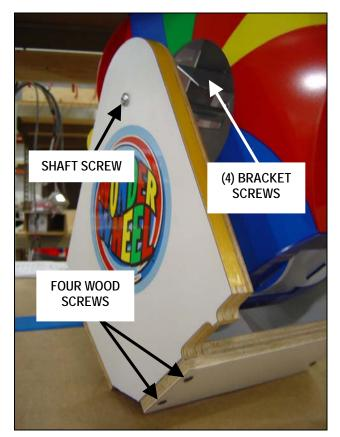
Figure 13 Wheel Disassembly
