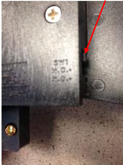
Coin Comparator Set to NC
