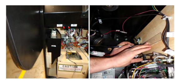
**STEP 2:** Where you just marked your holes install 2 Silver pan head screws but don't tighten all the way down (will need them to stick up about 1/16 of an inch for router to slide on)
