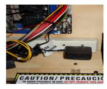
**STEP 7:** Plug in CEXXXX and Purple Network Cable cable into router and into MB8 PC board Both Cables MUST plug into the yellow sockets.
