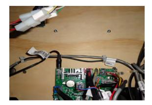
**STEP 3:** Unwrap and plug the power into the Wireless Router
